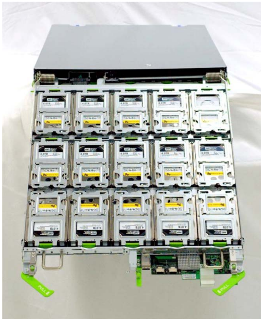
Figure 63 Front View of HDD Tray in Service
