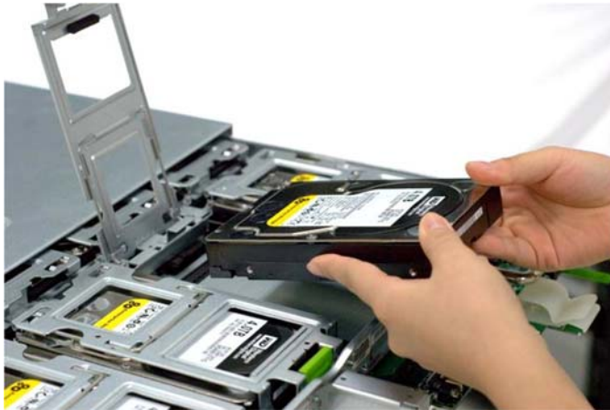
Figure 66 Hard Disk Drive Removal
