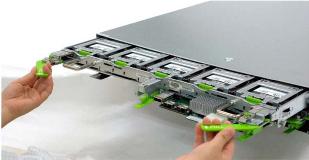
Figure 62 HDD Tray During Service
