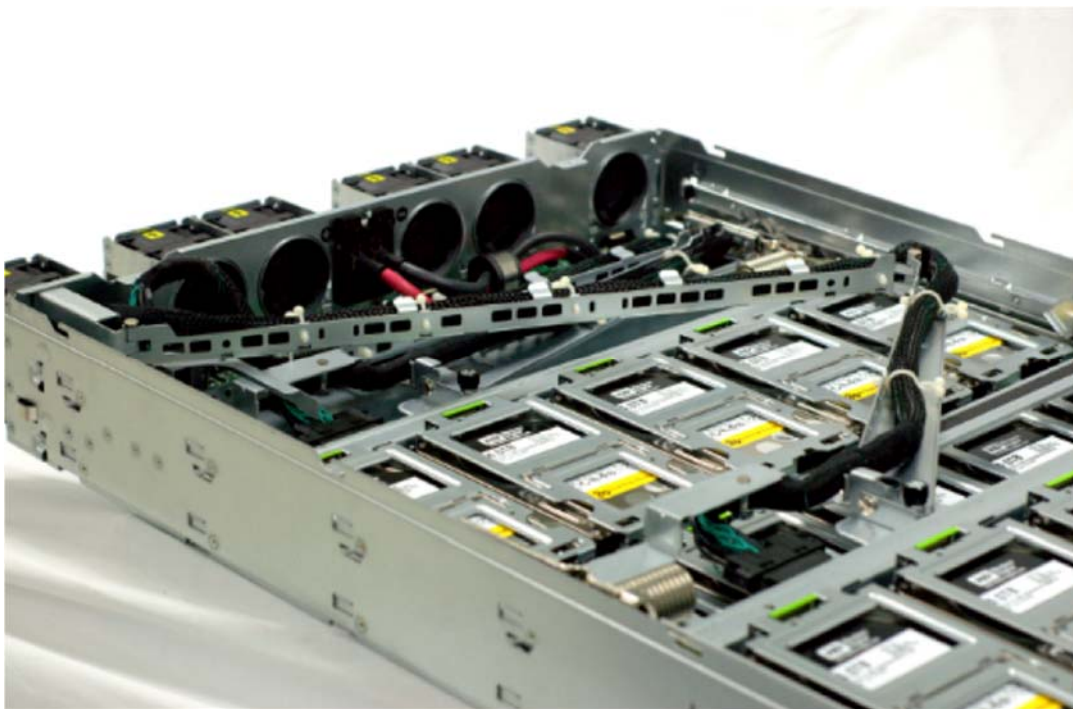
Figure 68 HDD Tray Cable Arm
