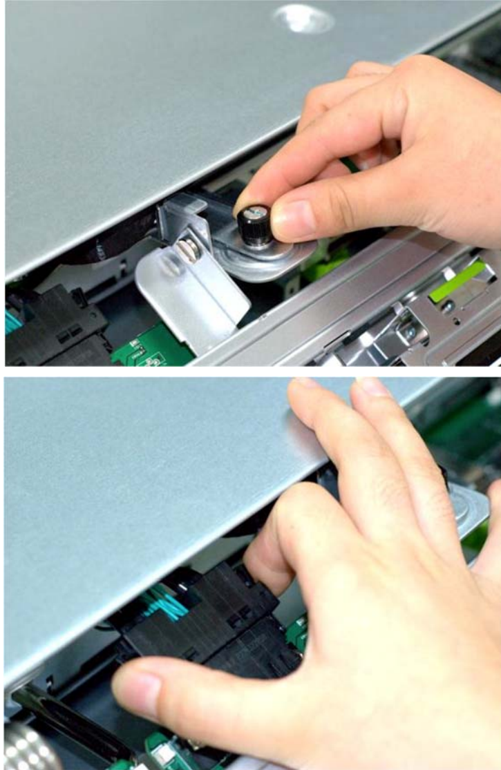
Figure 65 Cable Arm Release
