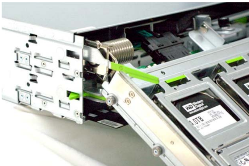
Figure 64 HDD Tray Release Lever
