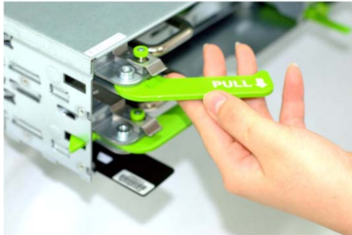
Figure 61 HDD Tray/Chassis Cam Latches
