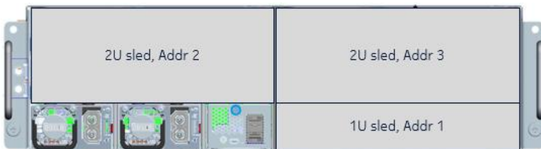
Figure 9 Open edge chassis with one 1U sled and two 2U sleds
