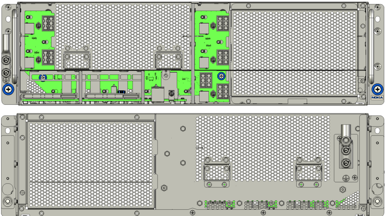
Figure 26 Chassis rear wall with backplane in place, front view (top), rear view (bottom)
