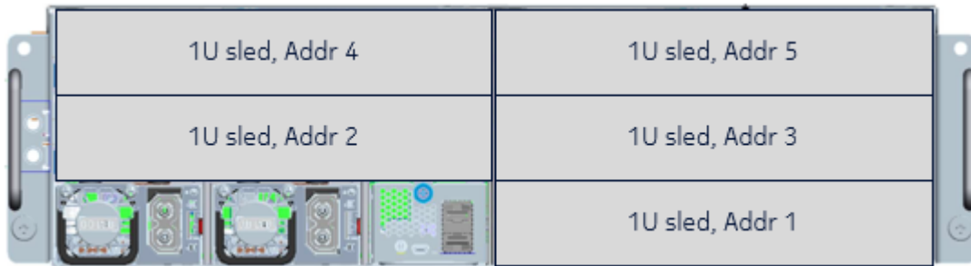
Figure 7 Open edge chassis with five 1U sleds
