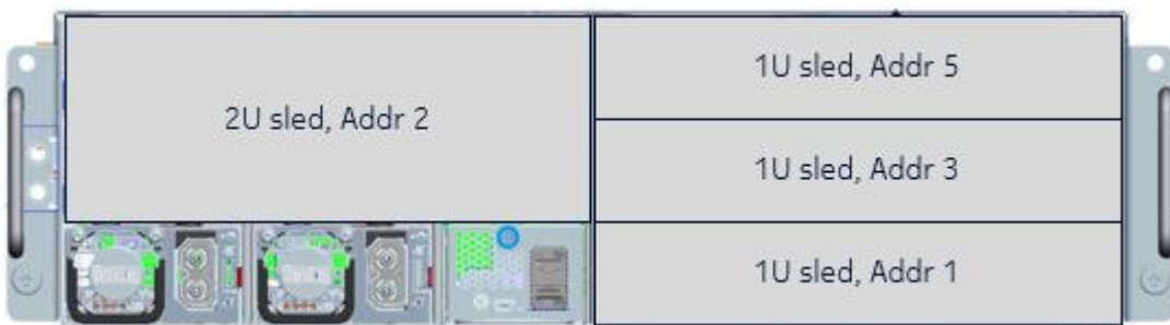
Figure 8 Open edge chassis with three 1U sleds and one 2U sled
