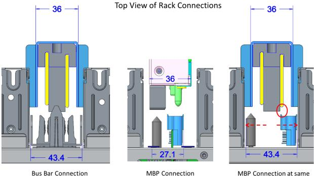
MBP Connection at same wider footprint as bus bar connector, if mistakenly installed at bus bar location
