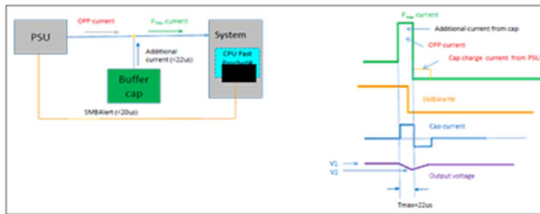
The total required Min buffer capacitance to support Pmax can be calculated as follows:
