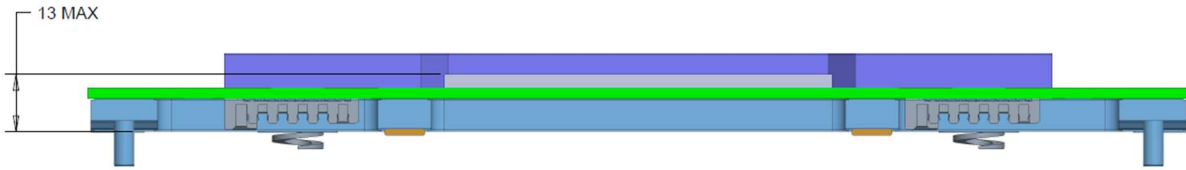
Figure 27 Maximum height of OAM to enable liquid cooling within a 1RU system
