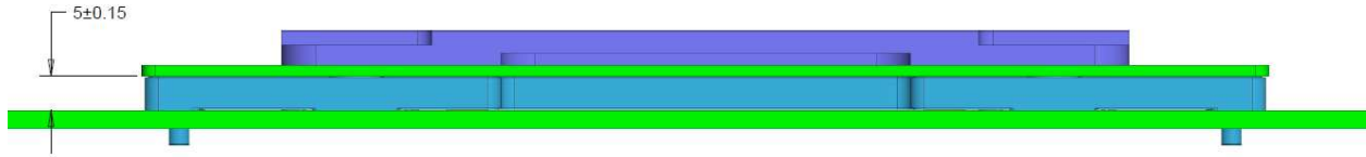
Figure 10 Tolerance Stack-up of Bottom Stiffener
