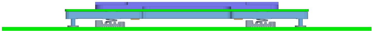
Figure 17 Side view (exploded) showing alignment pins being received by 1mm tall SMT nuts
