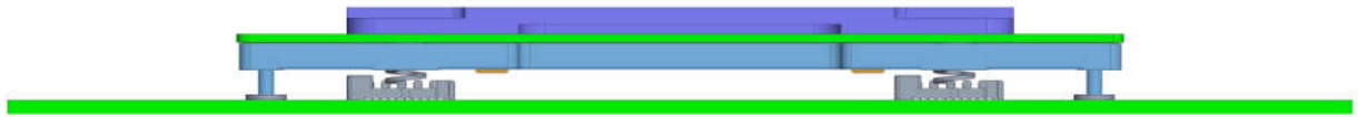
Figure 16 Side view (exploded) showing alignment pins being received by 1mm tall SMT nuts
