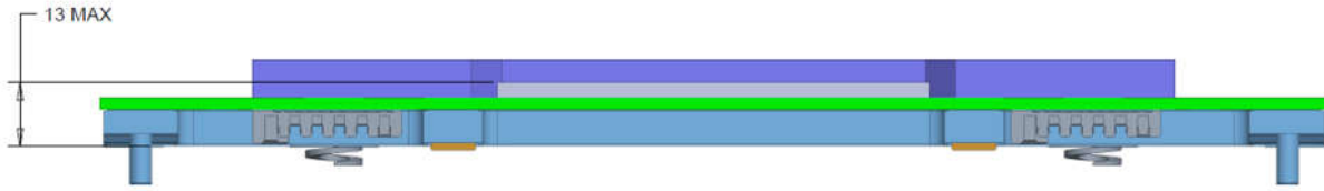
Figure 25 Maximum height of OAM to enable liquid cooling within a 1RU system
