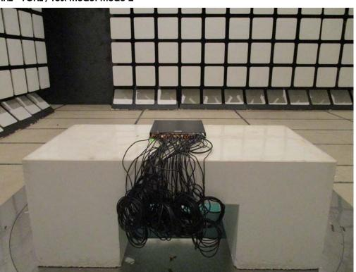
Test Configuration:  $30MHz \sim 1GHz$  / Test Mode: Mode 2
