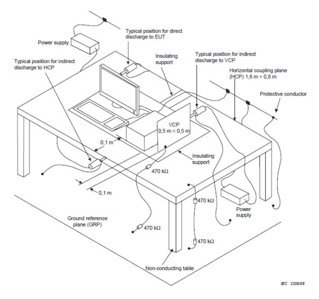
The test setup consists of the test generator, EUT and auxiliary instrumentation necessary to perform DIRECT and INDIRECT application of discharges to the EUT as applicable, in the follow manner: CONTACT DISCHARGE to the conductive surfaces and to coupling plane;
