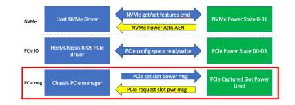
Ref: PCIe Base Specification 4.0 R1 Section 6.9 Slot Power Limit Control
