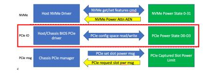
Ref: PCIe Base Specification 4.0 R1 Section 5.3 Device Power Management States (D-states) of a Function
