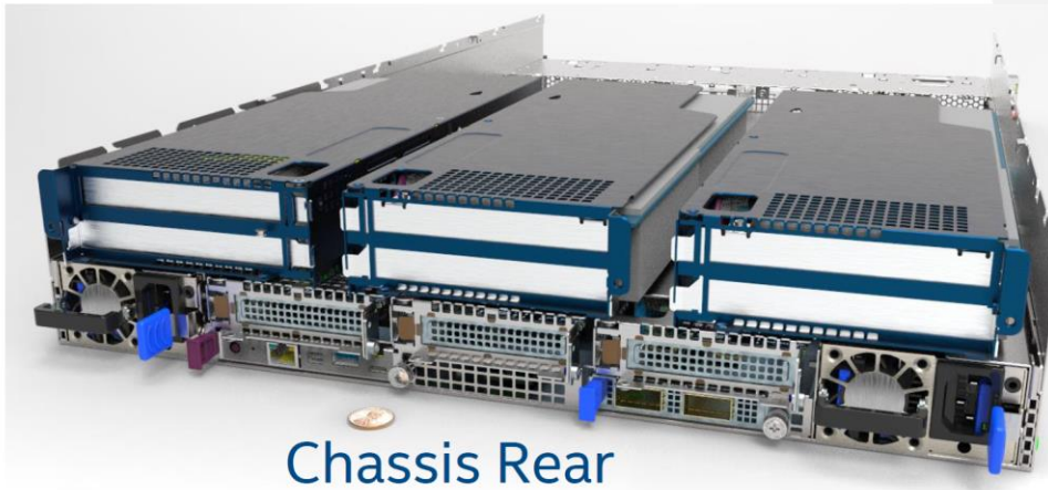
Figure 35. Examples of Typical 1U / 2U PCIe Slot Configs for Rear Management System
