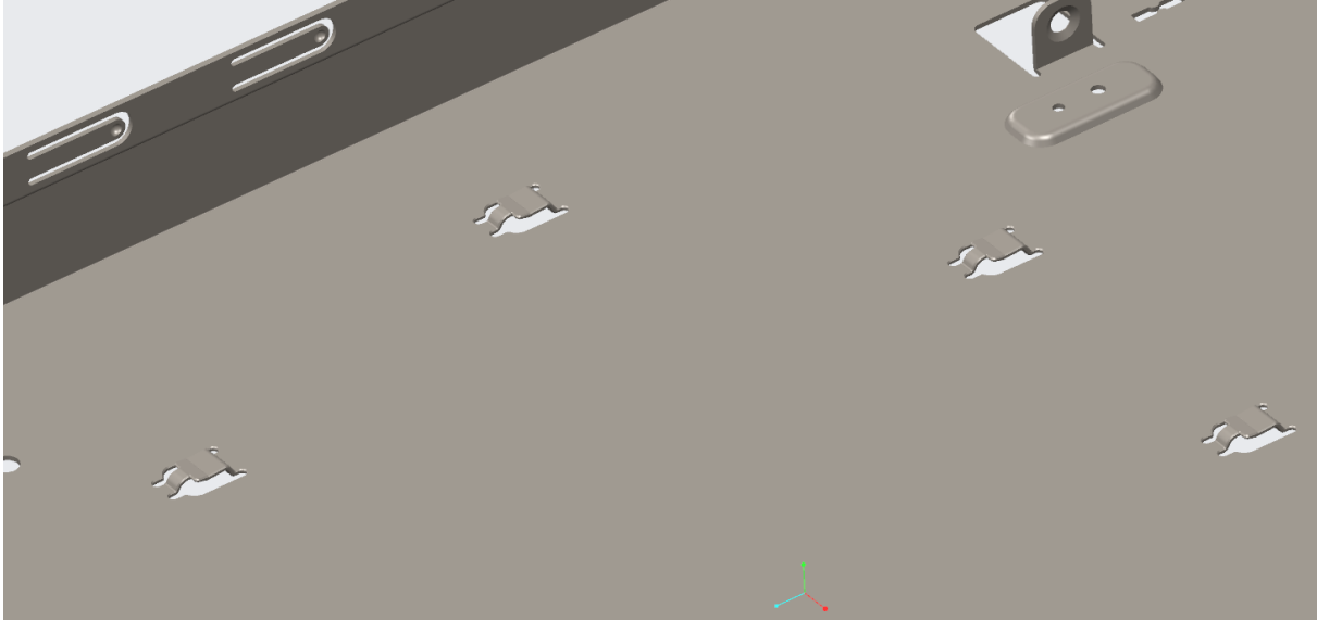
Figure 41. Example Chassis Base Geometry to Interface Chassis-to-Board Bracketry
