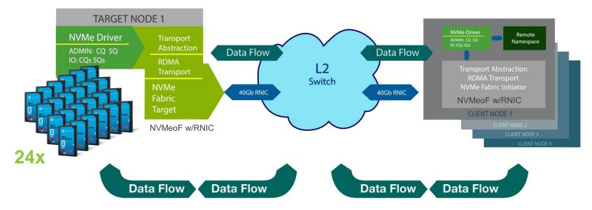
Data Flow bypassing target CPU
