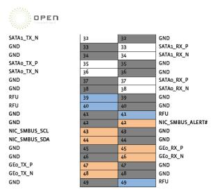
Figure 6-8 Pin Assignment Option 3, which Provides SATA and Ethernet Ports
