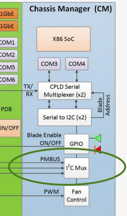
Chassis manager: fan control Variable fan speed based on blade requirements All blades polled for their PWM requirement Fan Control performed by the fan controller (ADT7470)
