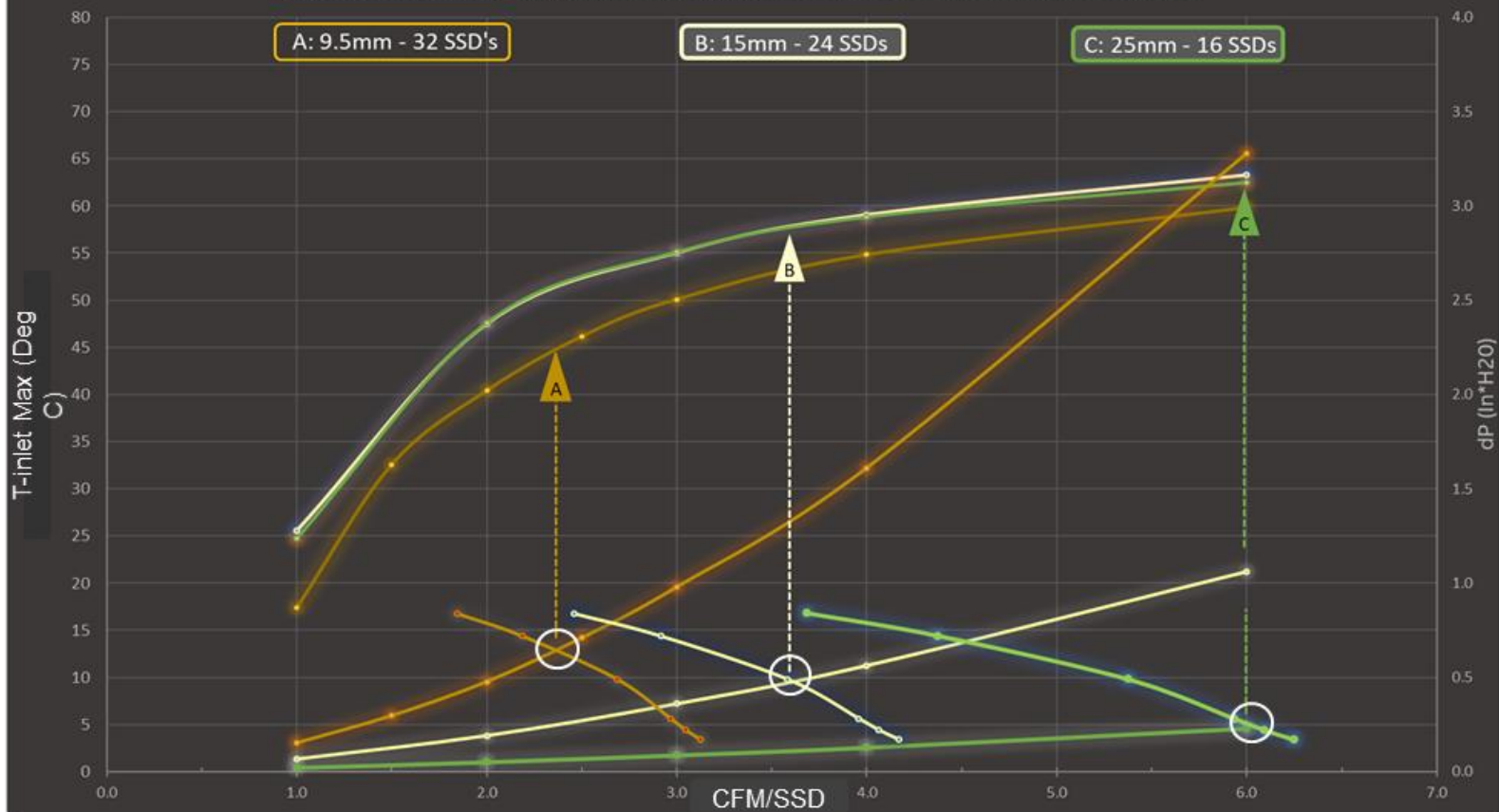
E1.S FF Comparison 9.5, 15, and 25mm Width @ 70% FSC Pseudo Fan Curves and 20W
