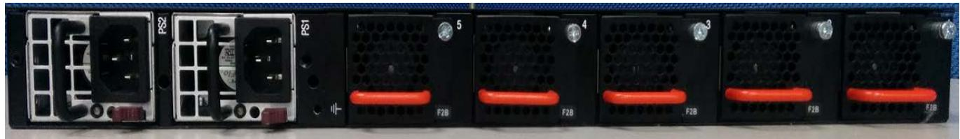
Redundant power supply modules
