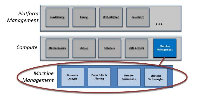
It is equally important to understand what Open Hardware Management is not. In this effort, we are making a distinction between Hardware Management and Platform Management. The Hardware Management effort is bounded by 1) the firmware on the machine, 2) event/alerting/logging about machine components and 3) basic remote management. Platform management encompasses all the other functions and is primarily about deploying and management operating systems and applications.
