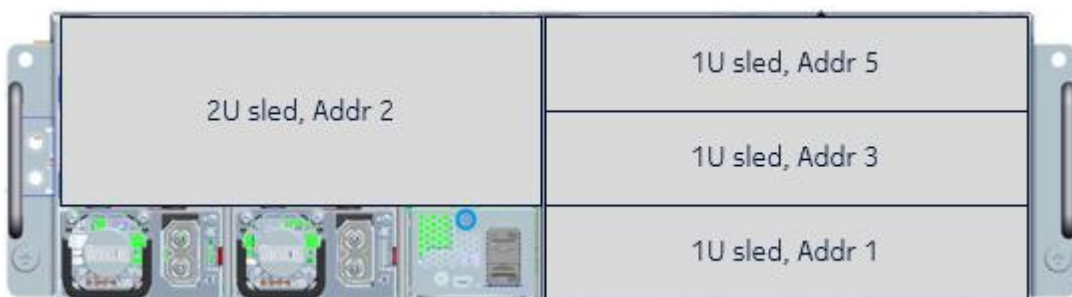
Figure 8 Open edge chassis with three 1U sleds and one 2U sled, option 1
