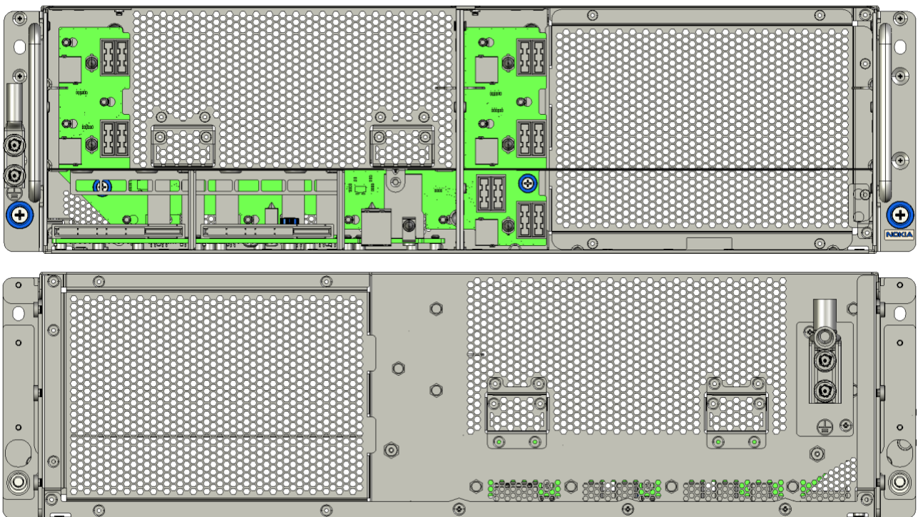
Figure 29 Chassis rear wall with backplane in place, front view (top), rear view (bottom)
