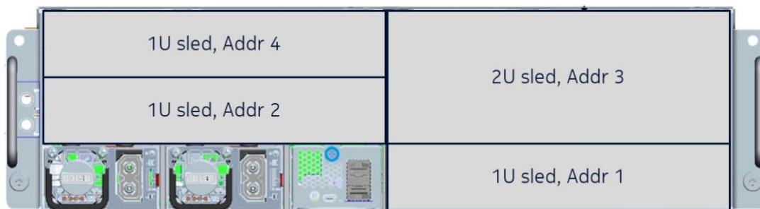
Figure 9 Open edge chassis with three 1U sleds and one 2U sled, option 2
