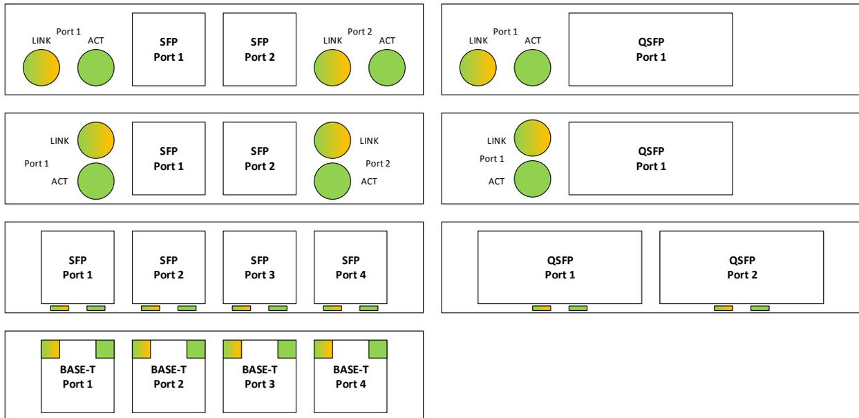
Note: The example port and LED ordering diagrams shown in Figure 89 are viewed with the card in the horizontal position and the primary side is facing up.
