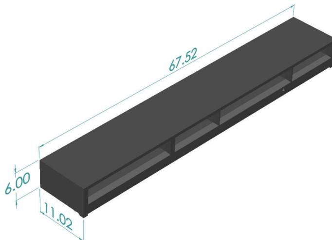
Figure 65: 140-pin Base Board Secondary Connector – Right Angle
