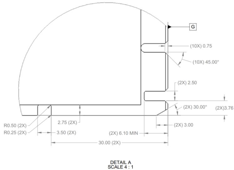
Figure 26: Small Form Factor Keep Out Zone – Bottom View
