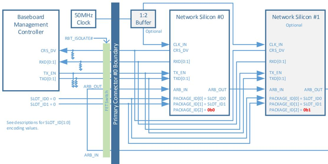
Figure 78: NC-SI Over RBT Connection Example – Dual Primary Connectors
