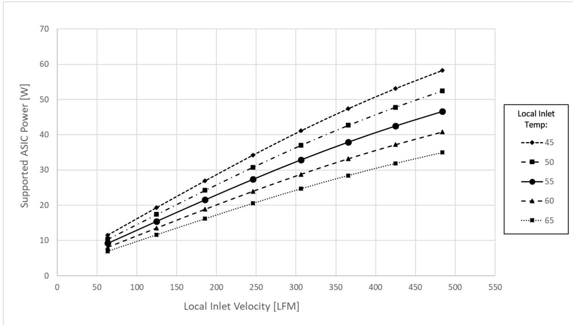
The curves shown in Figure 98 were obtained using CFD analysis of the reference OCP NIC 3.0 LFF card. The reference card has a 45mm x 45mm ASIC with two QSFP connectors. Additional card geometry parameters and boundary conditions used in the reference CFD analysis are summarized in Table 61. Figure 99 shows a comparison of the 3D CAD and CFD model geometry for the reference OCP NIC 3.0 card.
