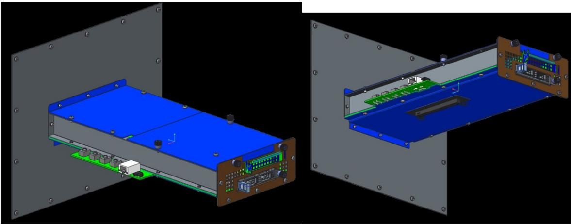
Figure 108: SFF Card Thermal Test Fixture Preliminary Design – Cover Removed
