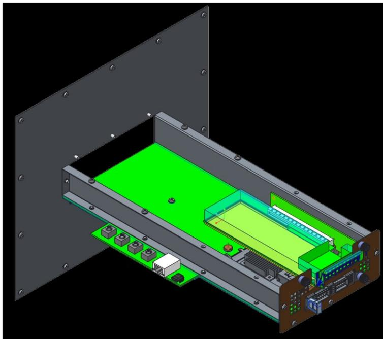
Figure 109: SFF Card Thermal Test Fixture PCB
