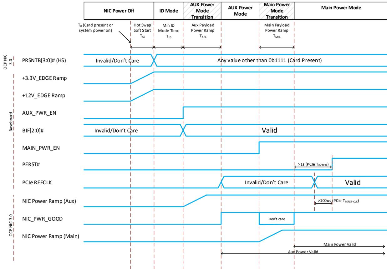
Figure 92: Power-Down Sequencing
