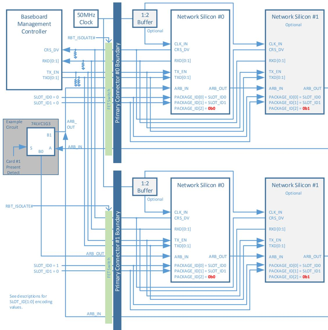
**Note 1:** For baseboard designs with a single Primary Connector, connect ARB\_IN to ARB\_OUT to complete the NC-SI hardware arbitration ring. For designs with multiple Primary Connectors, connect ARB\_IN and ARB\_OUT to an analog mux to complete the NC-SI arbitration ring based on the number of cards installed in the system. An example dual Primary Connector implementation is shown in Figure 78.
