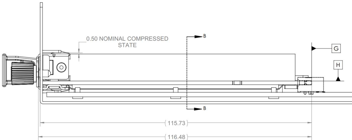
Figure 46: Small Form Factor Baseboard Chassis to Ejector lever Card CTF Dimensions (Side View)
