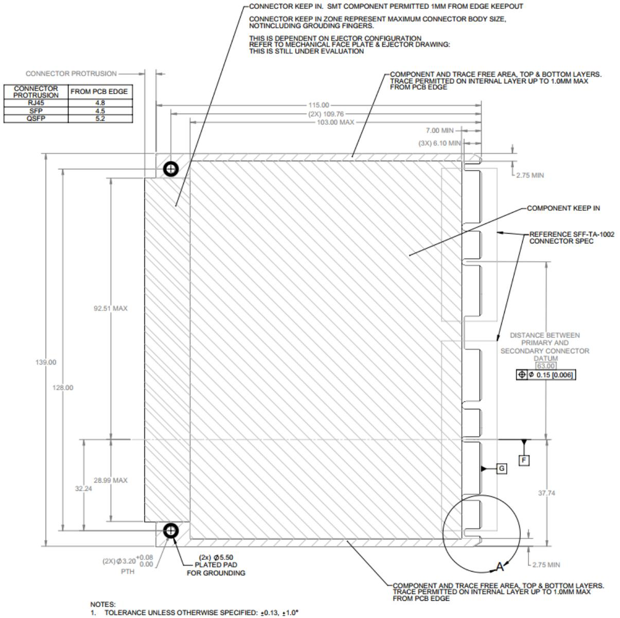
Figure 30: Large Form Factor Keep Out Zone – Top View – Detail A
