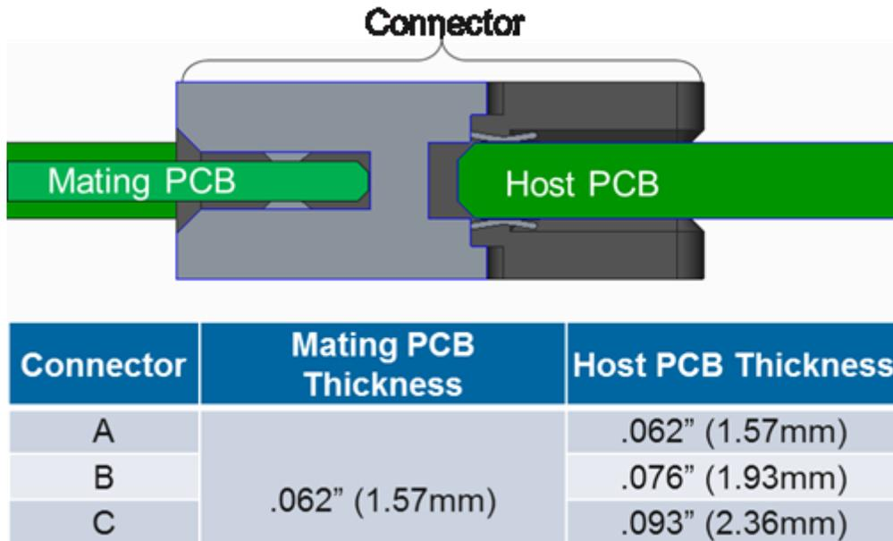
The connectors are capable of being used coplanar as shown in Figure 70. Additionally, the connectors are also capable of having a 0.3mm offset from the centerline of the host board as shown in Figure 71.
