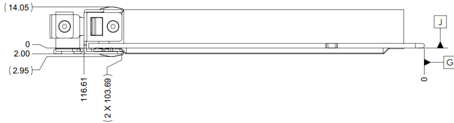
Figure 45: SFF OCP NIC 3.0 Card with Ejector CTF Dimensions (Side View)
