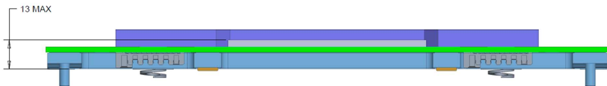
Figure 24 Maximum height of OAM to enable liquid cooling within a 1RU system
