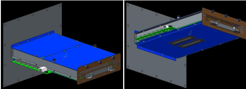
[Figure 137](#)~~136~~: LFF Card Thermal Test Fixture Design – Cover Removed
