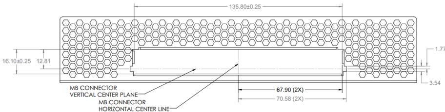
Figure 58: LFF Baseboard Chassis CTF Dimensions (Side View)
