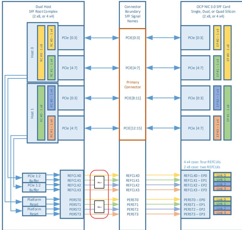
**Note:** For dual host applications that connect to a two link endpoint, the baseboard Host 1 REFCLK0 and PERST0 signal needs to be multiplexed to the REFCLK1 and PERST1 pins of the OCP NIC 3.0 card edge. This ensures the mandated Link n, REFCLKn and PERSTn mappings are maintained.
