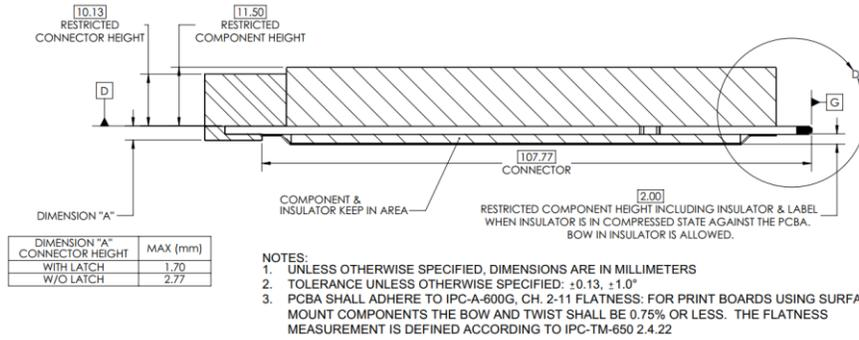
**Note:** The area defined by DIMENSION "A" is between the faceplate and the primary side of the board. Grounded through-hole mounting pins are permitted but should avoid making contact with the latching mechanism and EMI fingers. Signal pins are not permitted in this area.
