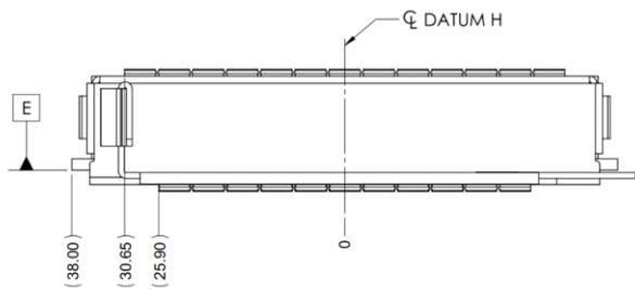
Figure 45: SFF OCP NIC 3.0 Card with Ejector CTF Dimensions (Side View)
