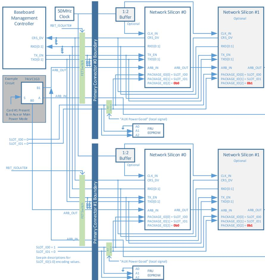
**Note 1:** For baseboard designs with a single Primary Connector, connect ARB\_IN to ARB\_OUT to complete the NC-SI hardware arbitration ring. For designs with multiple Primary Connectors, connect ARB\_IN and ARB\_OUT to an analog mux to complete the NC-SI arbitration ring based on the number of cards installed in the system. An example dual Primary Connector implementation is shown in Figure 86.
