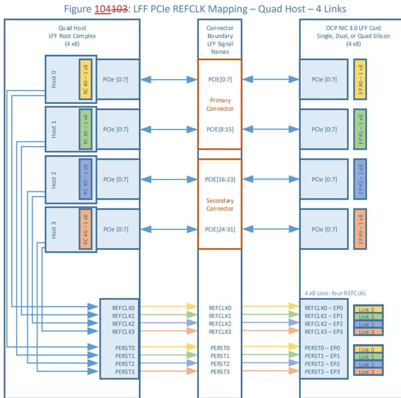
**Note:** For quad host applications that connect to a two link endpoint, the baseboard Host 2 REFCLK and PERST signal needs to be multiplexed to the REFCLK1 and PERST1 pins of the OCP NIC 3.0 card edge. This ensures the mandated Link  $n$ , REFCLK $n$  and PERST $n$  mappings are maintained.
