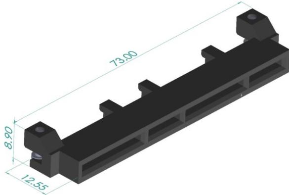
Figure 76: 140-pin Base Board Secondary Connector – Straddle Mount
