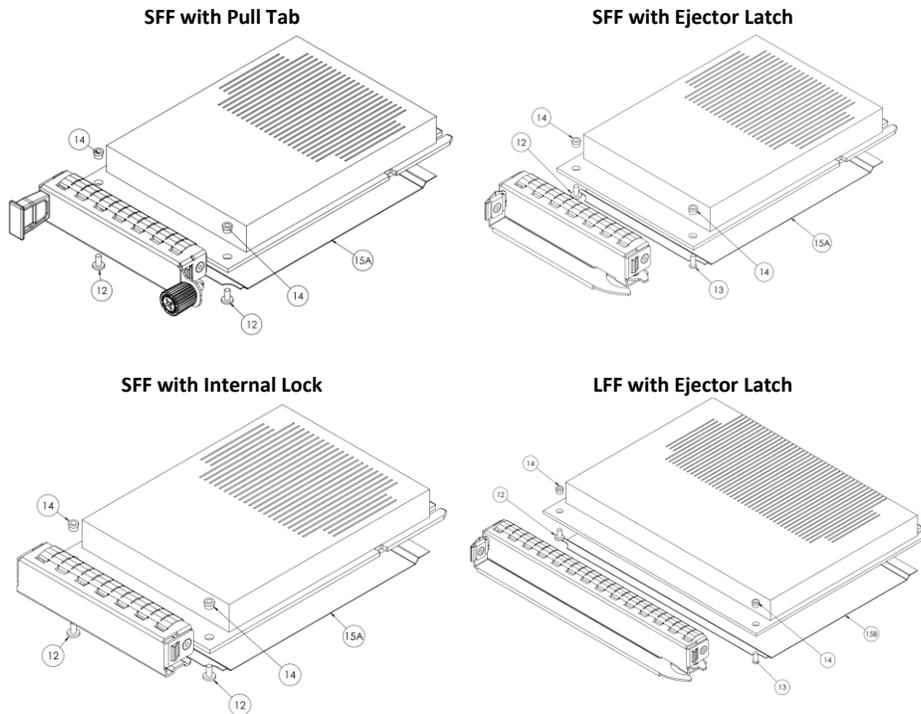
Diagram callouts #12 through #15 are installed at the NIC assembly level:
