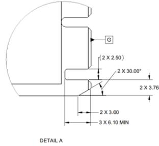
Figure 31: LFF Keep Out Zone – Bottom View
