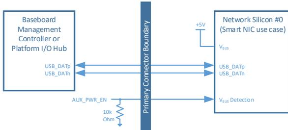
Figure 9294: USB 2.0 Connection Example – USB-Serial / USB-JTAG Connectivity
