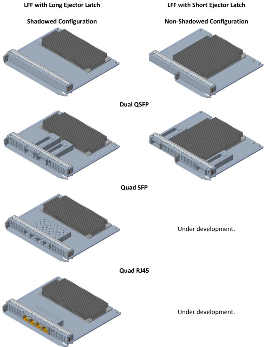
Figure 12 illustrates example LFF 3D views of the ejector latch assembly mounted in a chassis utilizing a straddle mount connector and a ~~right angle~~right-angle connector. The baseboard connector options are discussed in Section 3.2. The LFF OCP NIC 3.0 card is identical for both chassis connector options.
