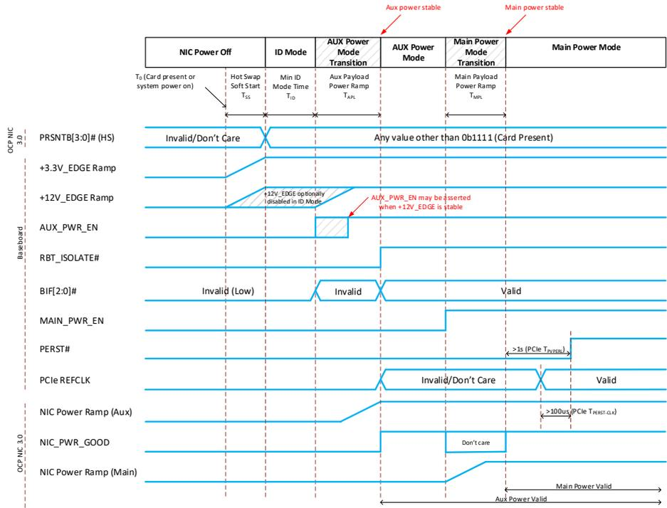
Note 1: The RBT isolation state is controlled with the baseboard RBT\_ISOLATE# signal. This controls the baseboard RBT isolator.
