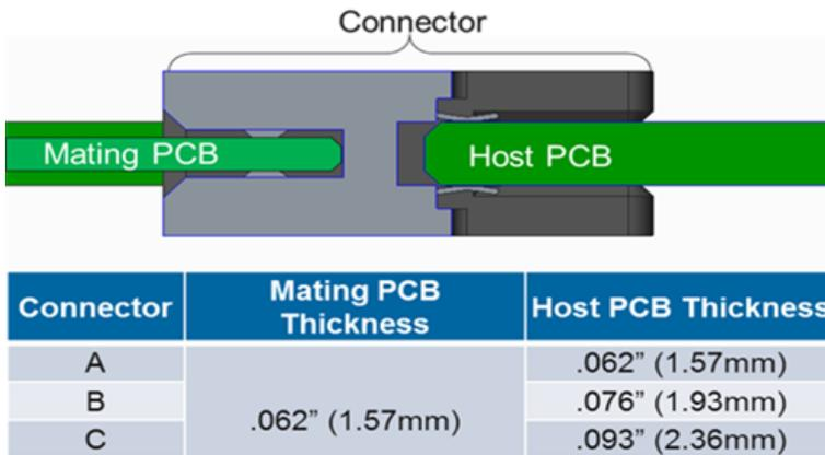
The connectors are capable of being used coplanar as shown in Figure 78. Additionally, the connectors are also capable of having a 0.3 mm offset from the centerline of the host board as shown in Figure 79.
