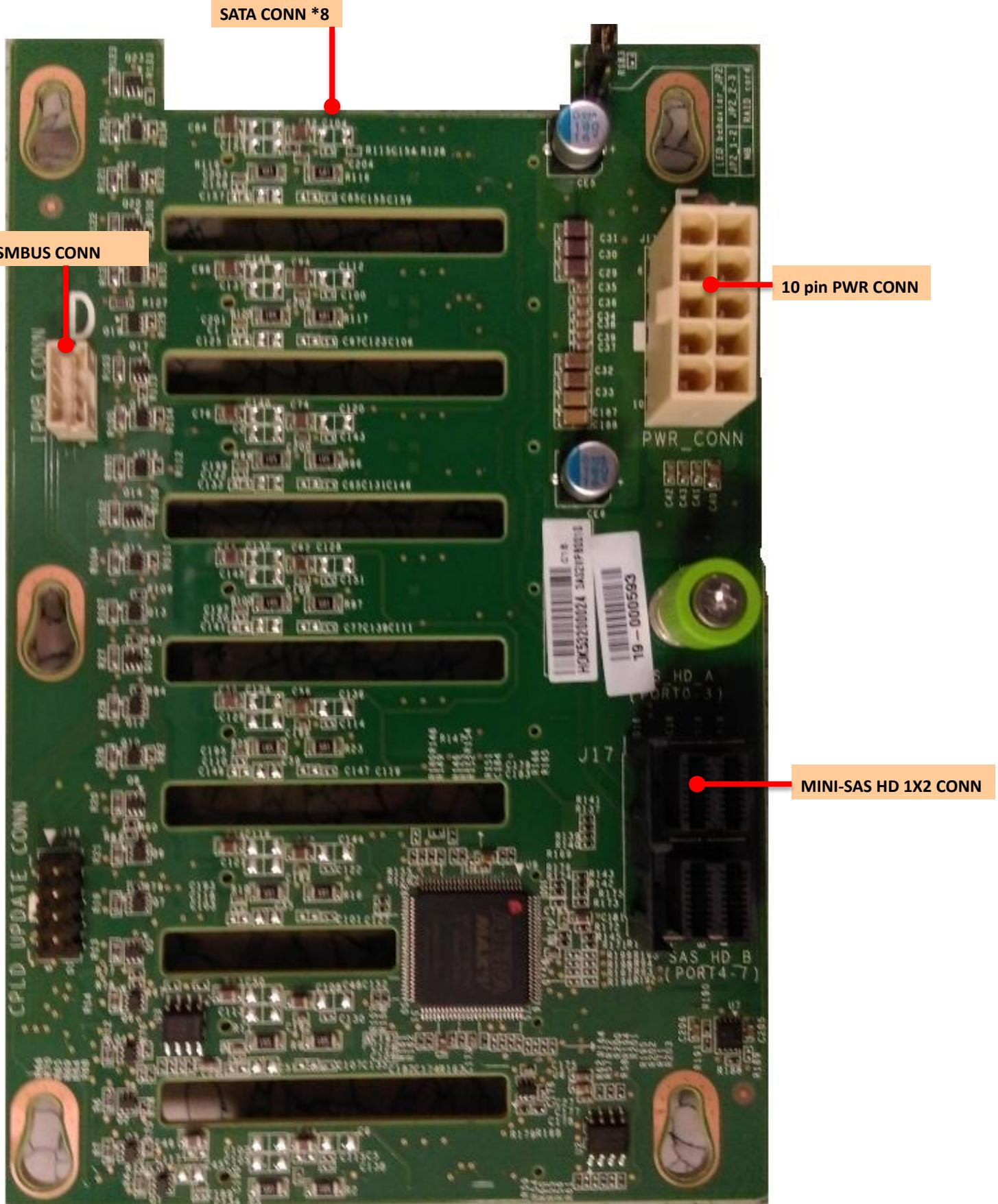
**Figure 3-7** HDD Backplane Board
