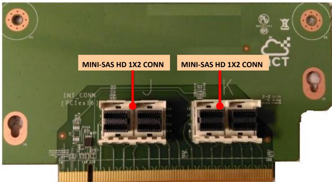
Figure 3-6 1x16 PCIE MINI-SAS HD Riser Board
