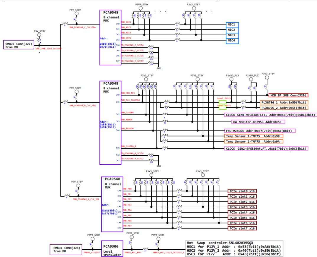
Figure 3-4 GPU Linking Board SMBUS Block Diagram
