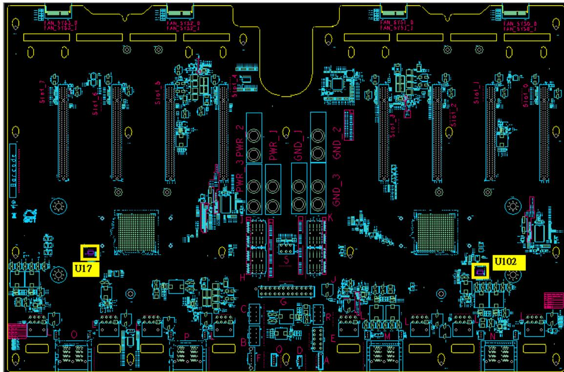
Figure 3-3 GPU Linking Board Temperature sensor location
