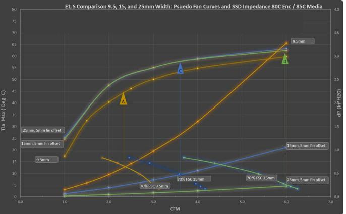
Trend: Increasing width achieves better system airflow, higher Tla, naturally achieves higher flow on the fan curve.
