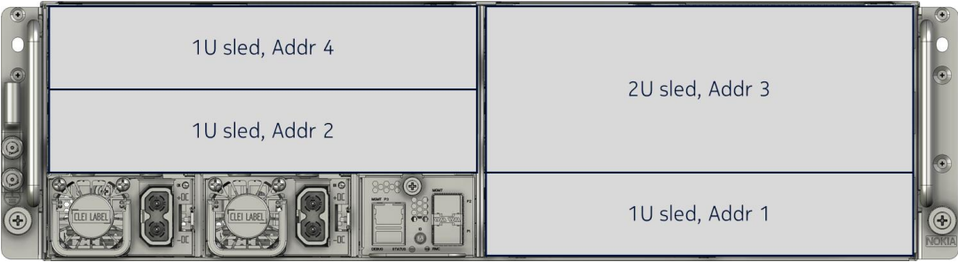
Figure 10 Open edge 3U chassis with three 1U sleds and one 2U sled, option 2
