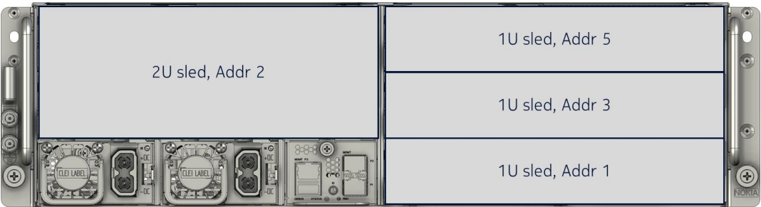
Figure 9 Open edge 3U chassis with three 1U sleds and one 2U sled, option 1
