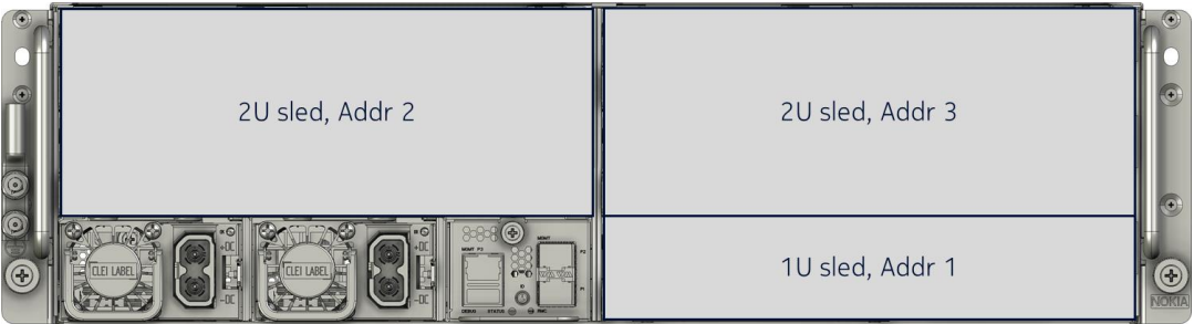
Figure 11 Open edge 3U chassis with one 1U sled and two 2U sleds
