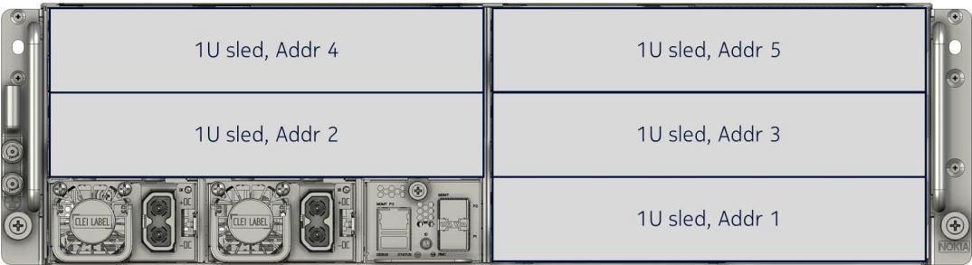
Figure 8 Open edge 3U chassis with five 1U sleds
