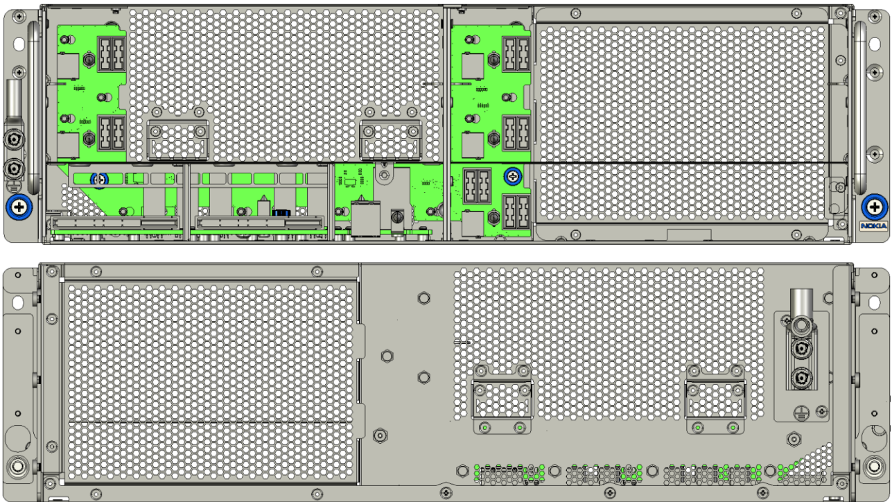
Figure 33 Chassis rear wall with backplane in place, front view (top), rear view (bottom)
