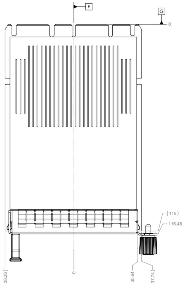
Figure 39: Small Form Factor OCP NIC 3.0 Card with Pull Tab CTF Dimensions (Front View)
