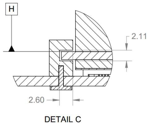
The right angle and straddle mount card guides are identical between the Small and Large form factor cards. The card guide model is included in the 3D CAD packages and may be downloaded from the OCP NIC 3.0 Wiki site: <http://www.opencompute.org/wiki/Server/Mezz>.
