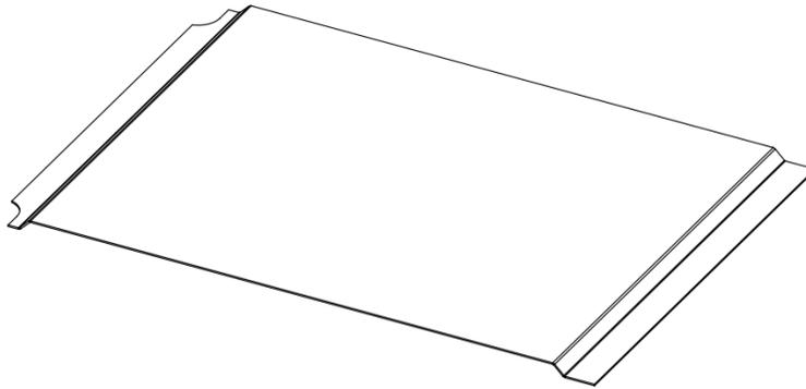
Figure 35: Small Card Bottom Side Insulator (Top and Side View)
