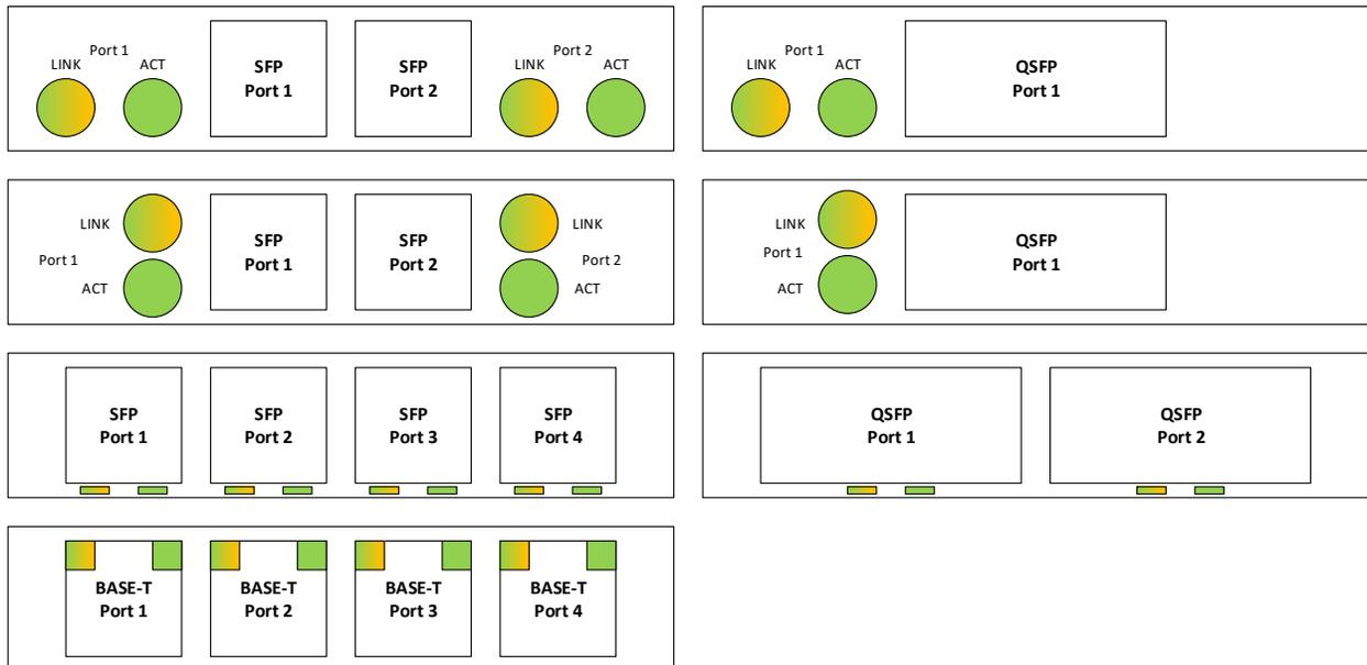
Note: The example port and LED ordering diagrams shown in Figure 92 are viewed with the card in the horizontal position and the primary side is facing up.
