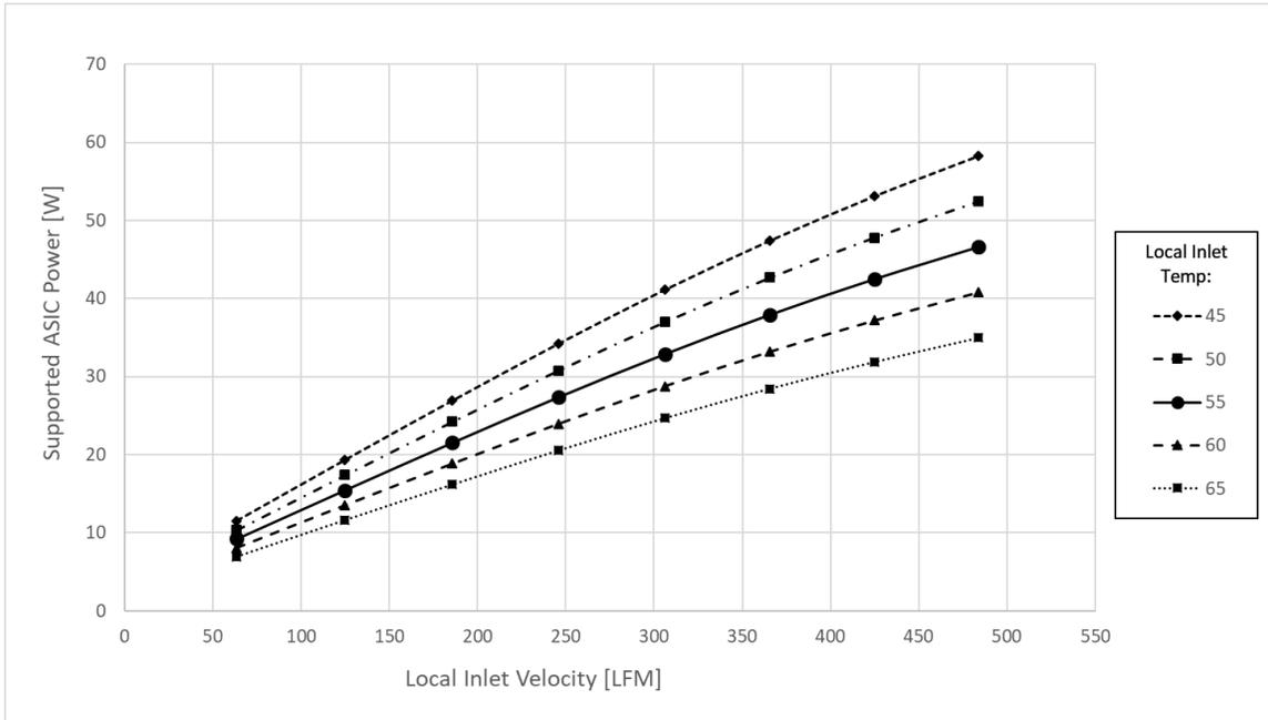
The curves shown in Figure 103 were obtained using CFD analysis of the reference OCP NIC 3.0 LFF card. The reference card has a 45mm x 45mm ASIC with two QSFP connectors. Additional card geometry parameters and boundary conditions used in the reference CFD analysis are summarized in Table 66. Figure 104 shows a comparison of the 3D CAD and CFD model geometry for the reference OCP NIC 3.0 card.
