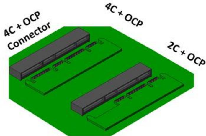
Table 5 summarizes the supported card form factors. Small form factors cards support the Primary Connector and up to 16 PCIe lanes. Large form factor cards support implementations with both the Primary and Secondary Connectors and up to 32 PCIe lanes, or a Primary Connector only implementation with up to 16 PCIe lanes.
