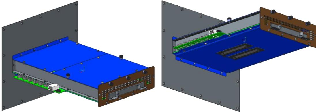
Figure 116: LFF Card Thermal Test Fixture Design – Cover Removed
