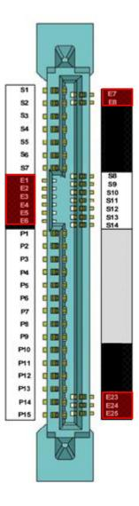
Eleven new pins on the U.3 SFF-8639 connector would be needed for a U.3 HDD: E1: REFCLKB+ E2: REFCLKB-E3: +3.3Vaux (used to supply SMBus EEPROM) E4: PERSTB# E5: PERST# E6: IFDet2# E7: REFCLK+ E8: REFCLK+ E8: REFCLK-E23: SMBCLK E24: SMBDAT E25: DualPortEn#
