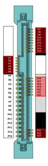
Twenty-five new pins on the U.2 SFF-8639 connector potentially would be needed for a U.2-HDD: E1: REFCLKB+ E2: REFCLKB-E3: +3.3Vaux (used to supply SMBus EEPROM) E4: PERSTB# E5: PERST# E6: IFDet2# E7: REFCLK+ E8: REFCLK+ E9-E15: PCIe Port 0 E23: SMBCLK E24: SMBDAT E25: DualPortEn# S16-S22: PCIe Port 1
