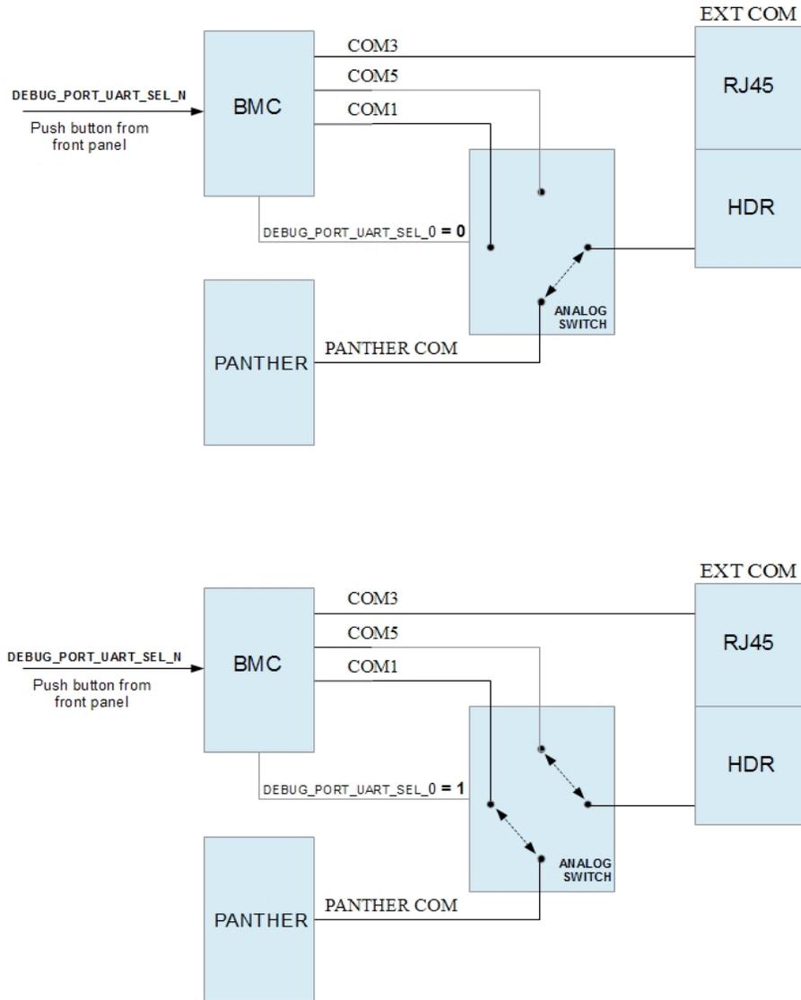
Figure 21: Debug port switching
