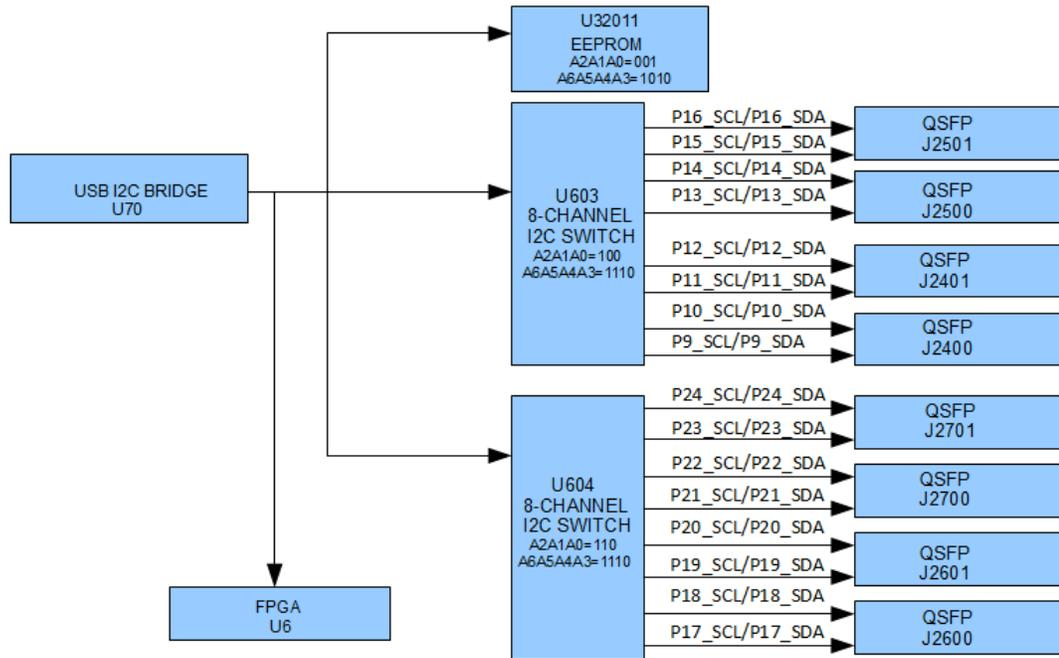
Figure 27: Micro Server I2C access to QSFP
