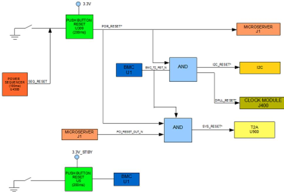
Figure 26: Reset Architecture
