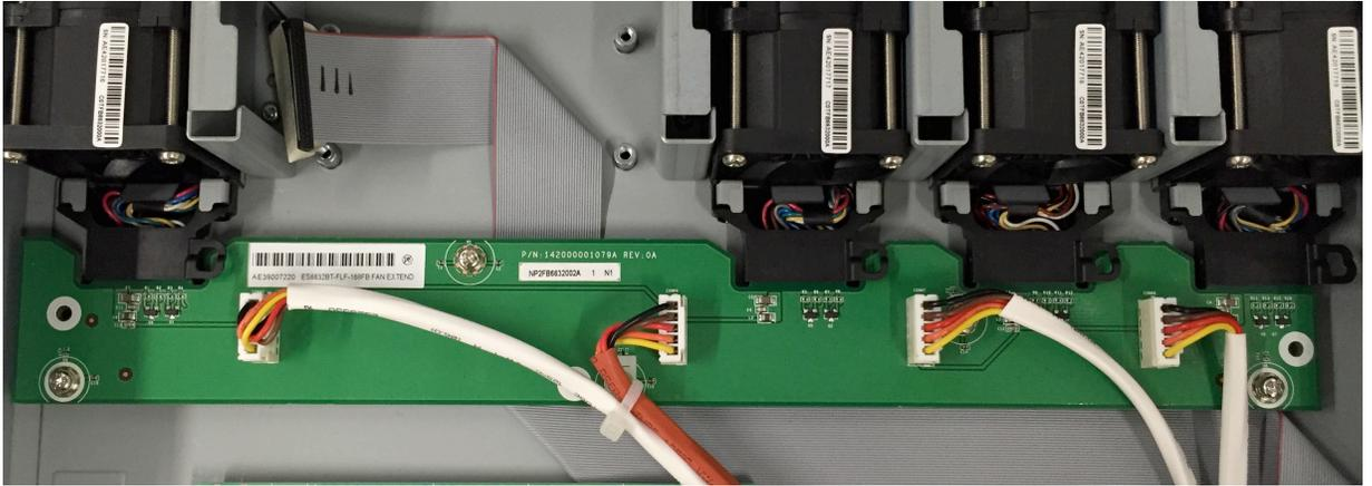
Figure 5: Fan Module
