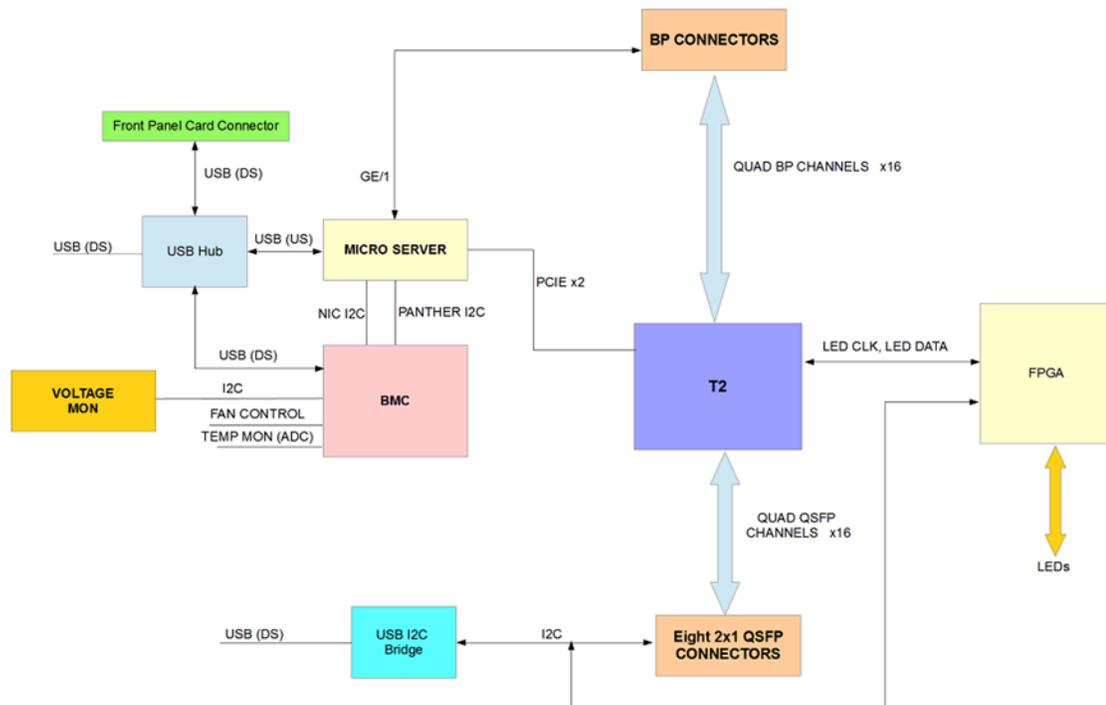
Figure 11: Main Switching Module Hardware Architecture
