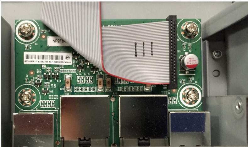
Figure 6: Rear Extension Module
