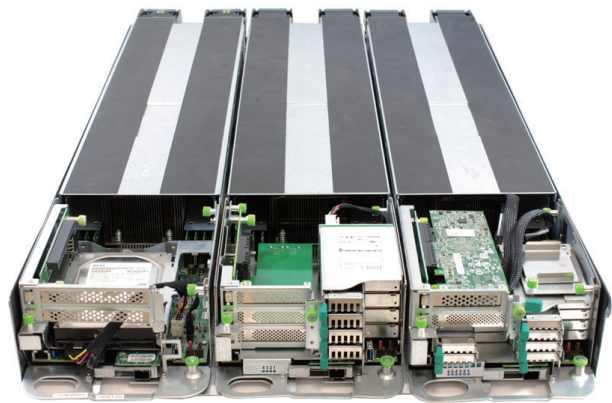
Three Wiwynn SV7220G2 servers in a 2OU (Open Rack) space
