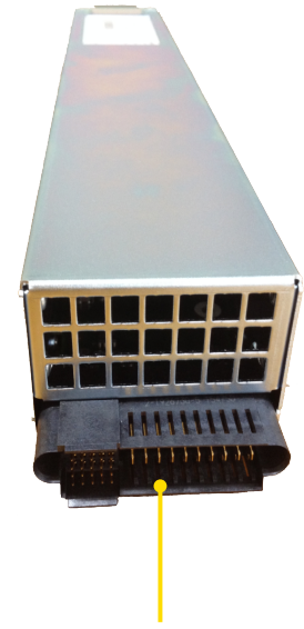
12V power to wedge-100 main board
