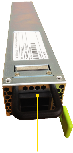
12V bus bar power input connector
