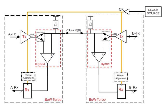
A Hybrid block, placed between the pad and basic BoW Tx/Rx ports, creates a Bow Turbo port
