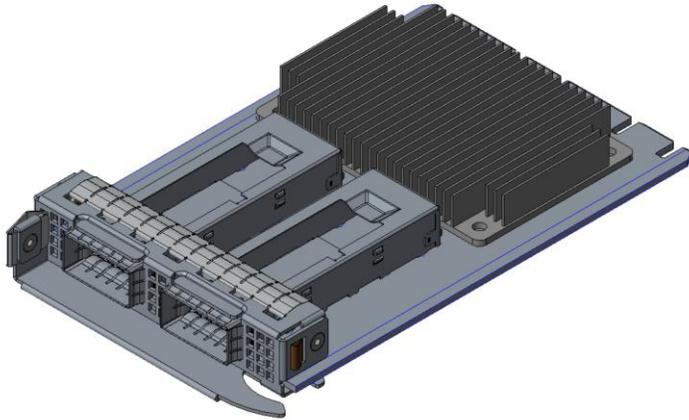
Note: The OCP NIC 3.0 card supplier shall add port identification on the bracket that meet their manufacturing and customer requirements.
