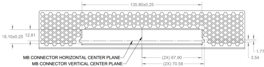
Figure 37: Large Form Factor Baseboard Chassis CTF Dimensions (Side View)
