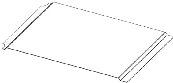
Figure 52: Small Card Bottom Side Insulator (Top and Side View)
