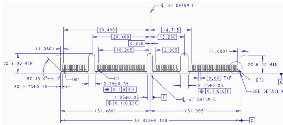
Figure 64: Large Size Card Gold Finger Dimensions – x32 – Top Side (“B” Pins)
