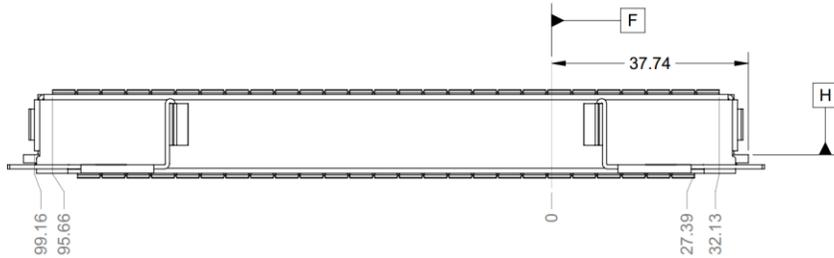
Figure 35: Large Form Factor OCP NIC 3.0 Card with Ejector CTF Dimensions (Side View)
