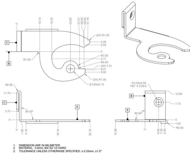
Figure 30: Large Card Standard I/O Bracket – Right Ejector Lever
