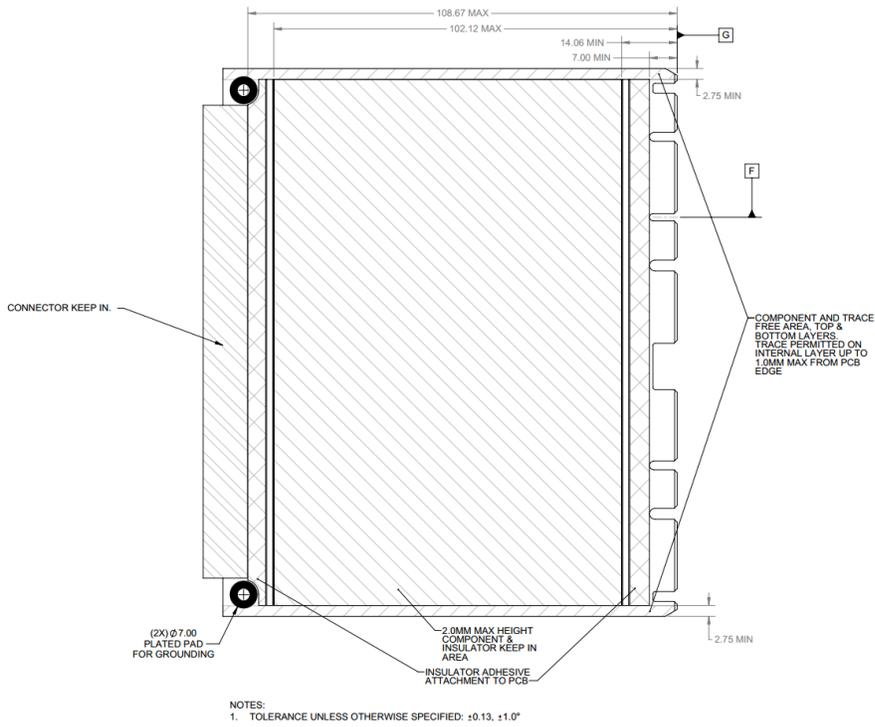
Figure 49: Large Form Factor Keep Out Zone – Side View
