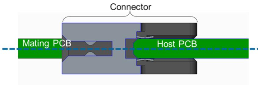
Figure 73: 0.3mm Offset for 0.076" Thick Baseboards
