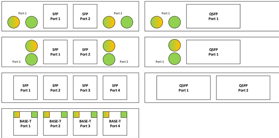
Note: The example port and LED ordering diagrams shown in Figure 40 are viewed with the card in the horizontal position and the primary side is facing up.
