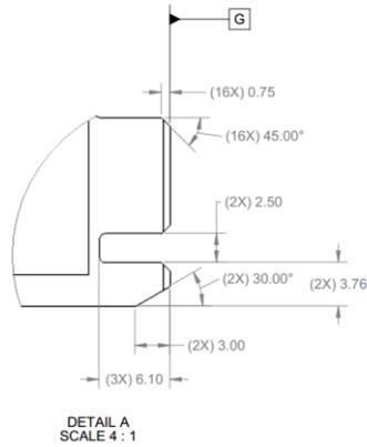
Figure 48: Large Form Factor Keep Out Zone – Bottom View
