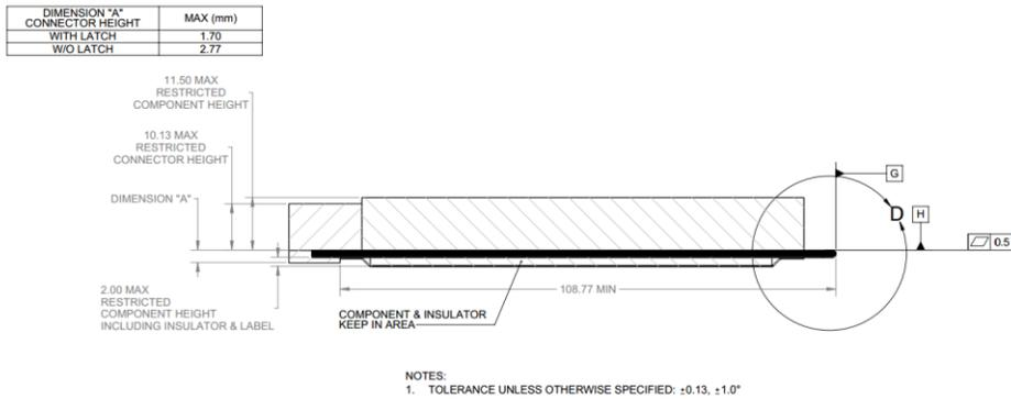
Figure 45: Small Form Factor Keep Out Zone – Side View – Detail D
