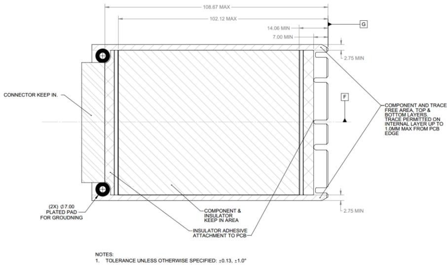
Figure 44: Small Form Factor Keep Out Zone – Side View
