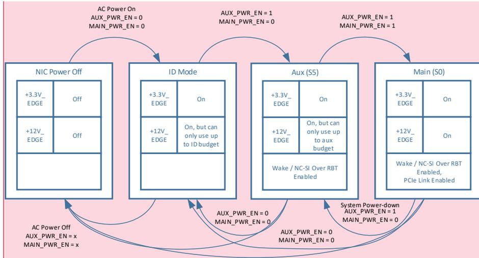
**Commented [NT4]:** For 0v80, a more formal definition of the power state diagram needs to be drawn. This will include the transition delay times from ID-AUX and AUX-MAIN.
