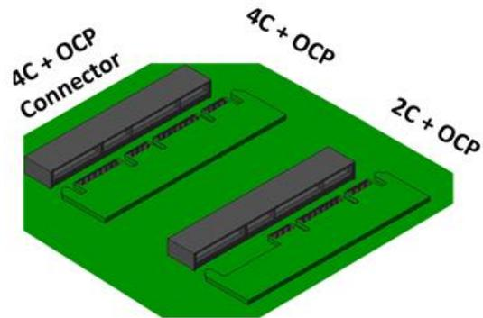
Table 4 summarizes the supported card form factors. Small form factors cards support the Primary Connector and up to 16 PCIe lanes. Large form factor cards support implementations with both the Primary and Secondary Connectors and up to 32 PCIe lanes, or a Primary Connector only implementation with up to 16 PCIe lanes.
