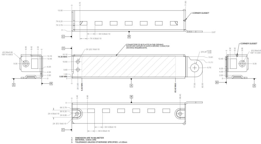
Figure 11 shows the Small Card form factor ejector lever.
