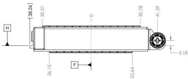
Figure 18: Small Form Factor OCP NIC 3.0 Card with Thumbscrew CTF Dimensions (Side View)
