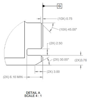
Figure 43: Small Form Factor Keep Out Zone – Bottom View
