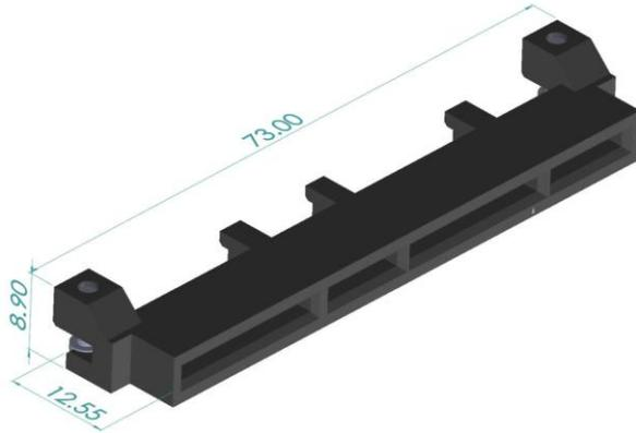
Figure 70: 140-pin Base Board Secondary Connector – Straddle Mount
