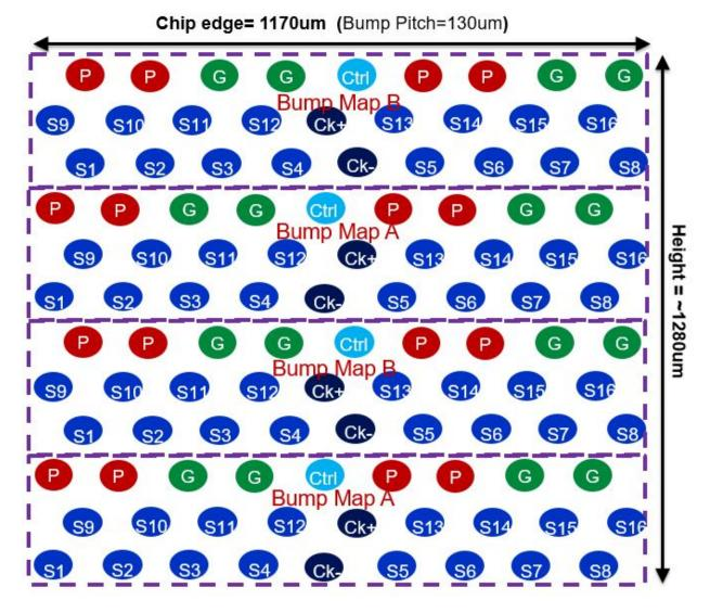
Example Bump Pattern (based on 130 um staggered bump pitch) shown below:
