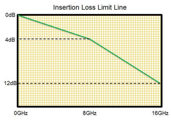
BoW channel limit is limited by the round trip reflection delay and limited to <10mm for a 5Gbaud with proper slew rate control
