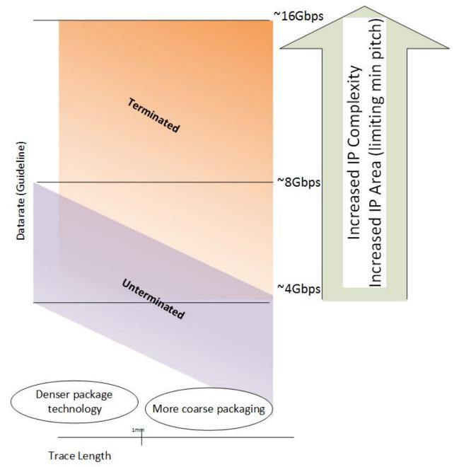
A high level view of the BoW Interface Data-rate ranges is shown below:
