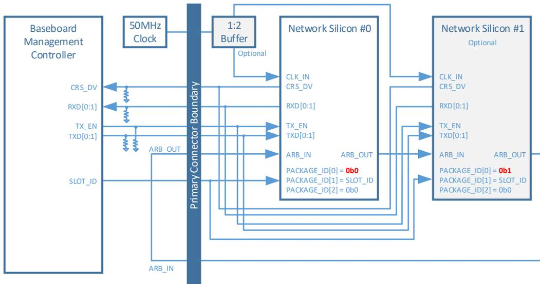
Figure 80: NC-SI Over RBT Connection Example – Dual Primary Connector
