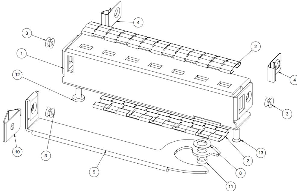
Figure 10: Small Card Generic I/O Bracket with a Latching Lever (2D View)
