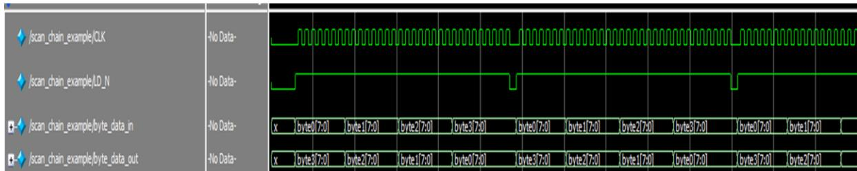
The scan chain provides side band status indication between the OCP NIC 3.0 card and the baseboard. The scan chain bit definition is defined in the two tables below. The scan chain data stream is 32-bits in length for both the DATA\_OUT and the DATA\_IN streams. The scan chain implementation is optional on the host, but is mandatory on all OCP NIC 3.0 cards. The scan chain components operates on the +3.3V\_EDGE power domain.
