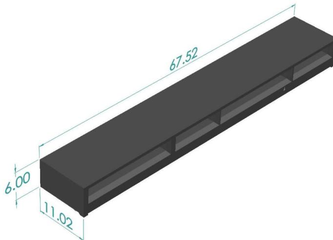
Figure 67: 140-pin Base Board Secondary Connector – Right Angle
