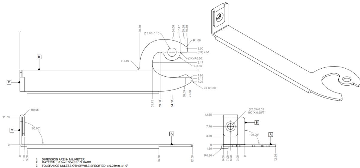
The Small Card ejector uses a locking mechanism at the end of the handle to retain the lever position. This is shown in Figure 12.
