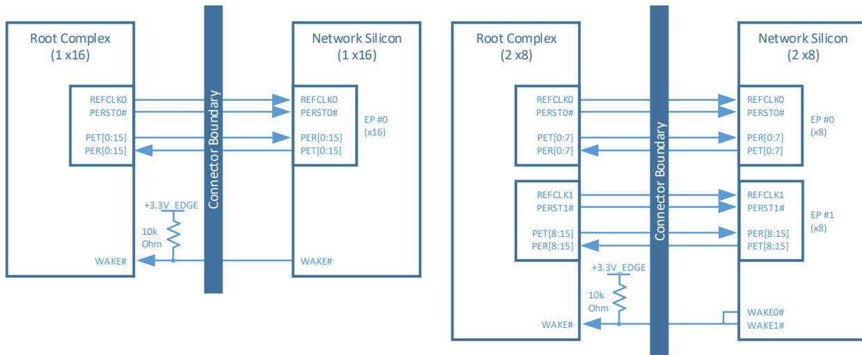
Figure 89: PCIe Interface Connections for a 4 x4 OCP NIC 3.0 Card
