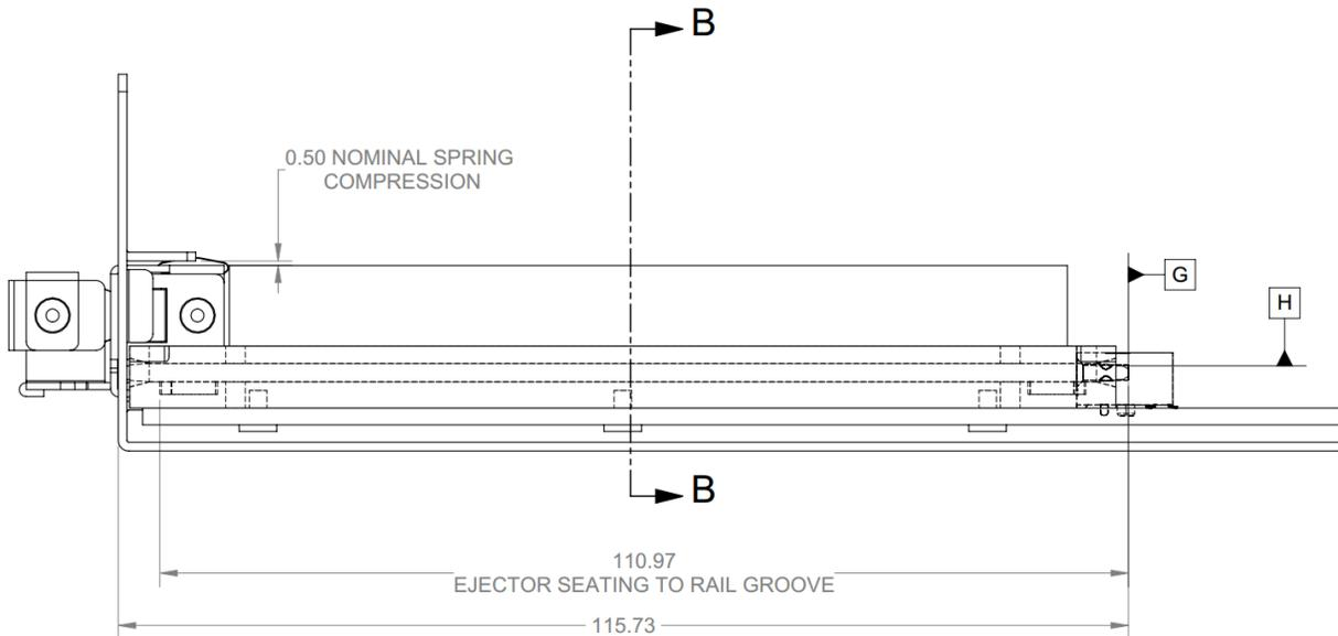
Figure 25: Small Form Factor Baseboard Chassis CTF Dimensions (Rear Rail Guide View)
