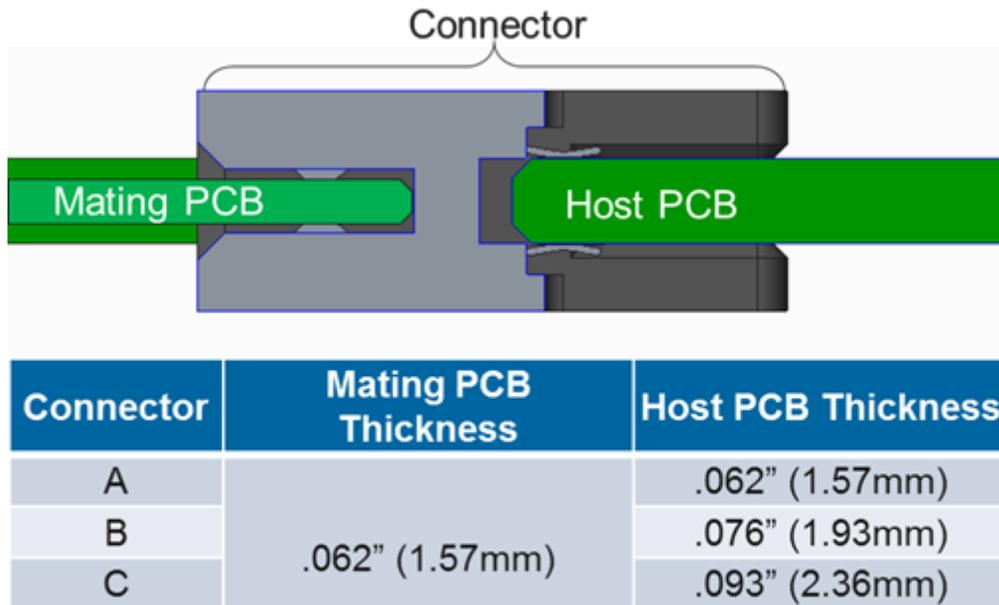
The connectors are capable of being used coplanar as shown in Figure 72. Additionally, the connectors are also capable of having a 0.3mm offset from the centerline of the host board as shown in Figure 73.
