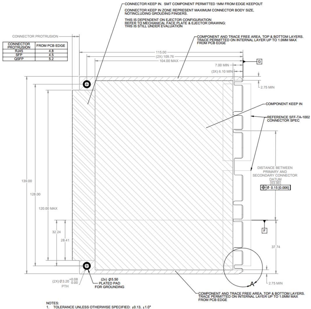
Figure 47: Large Form Factor Keep Out Zone – Top View – Detail A
