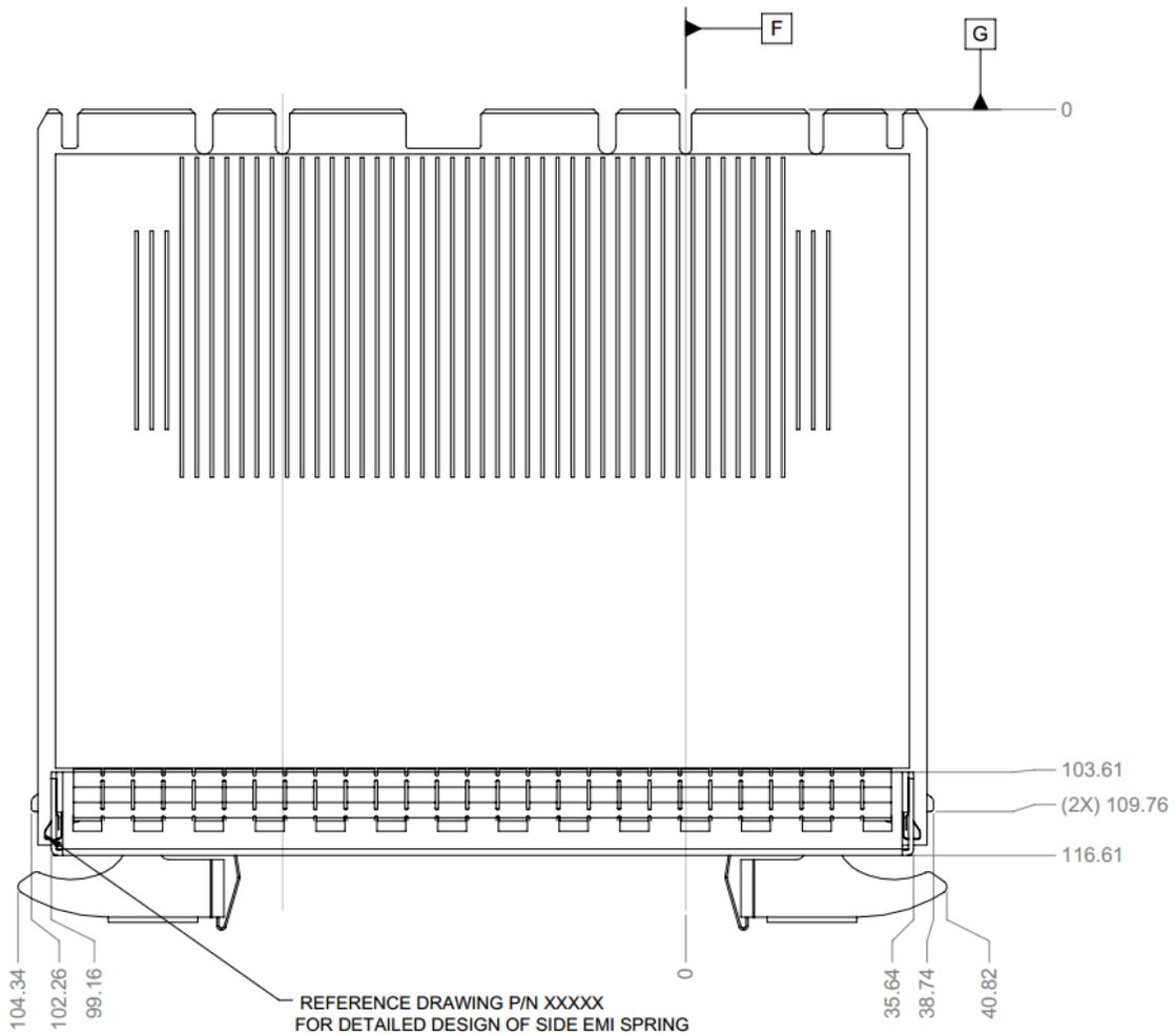
Figure 34: Large Form Factor OCP NIC 3.0 Card with Ejector CTF Dimensions (Front View)
