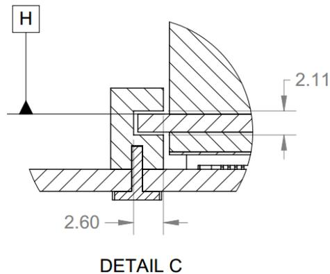
Card guides are identical between the Small and Large form factor cards. The card guide 3D CAD packages may be downloaded from the OCP NIC 3.0 Wiki site:
