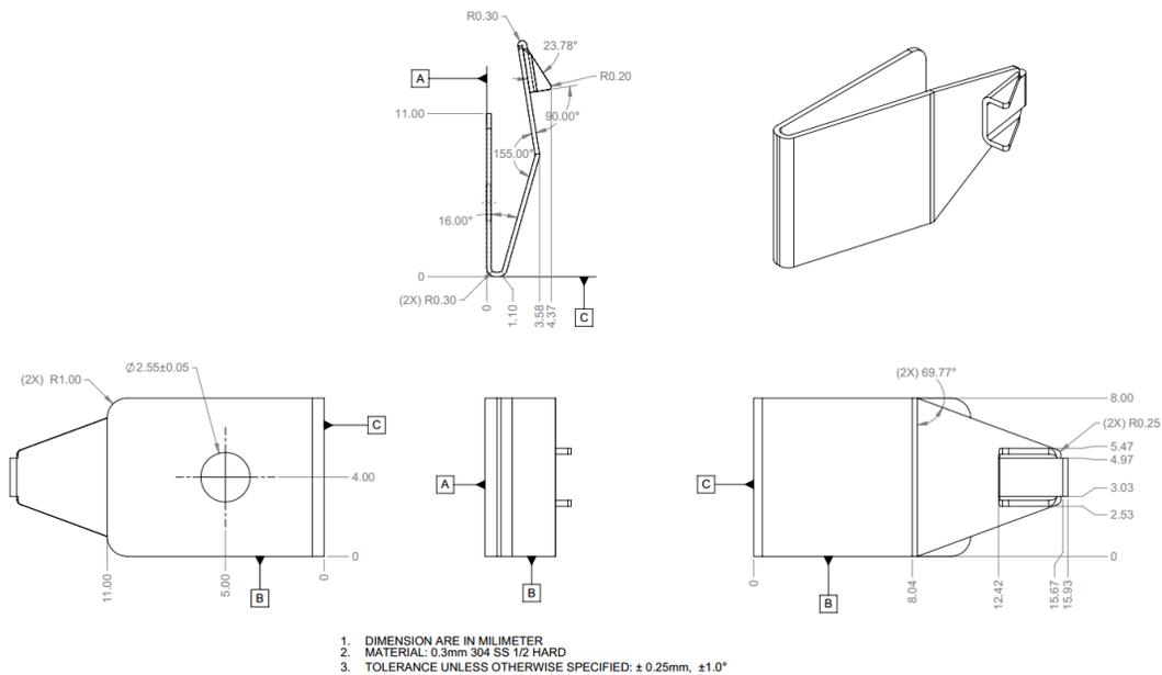
The side EMI finger is defined in Figure 13. The top and bottom EMI fingers are commercial off the shelf components and are listed in the mechanical BOM in Table 5.
