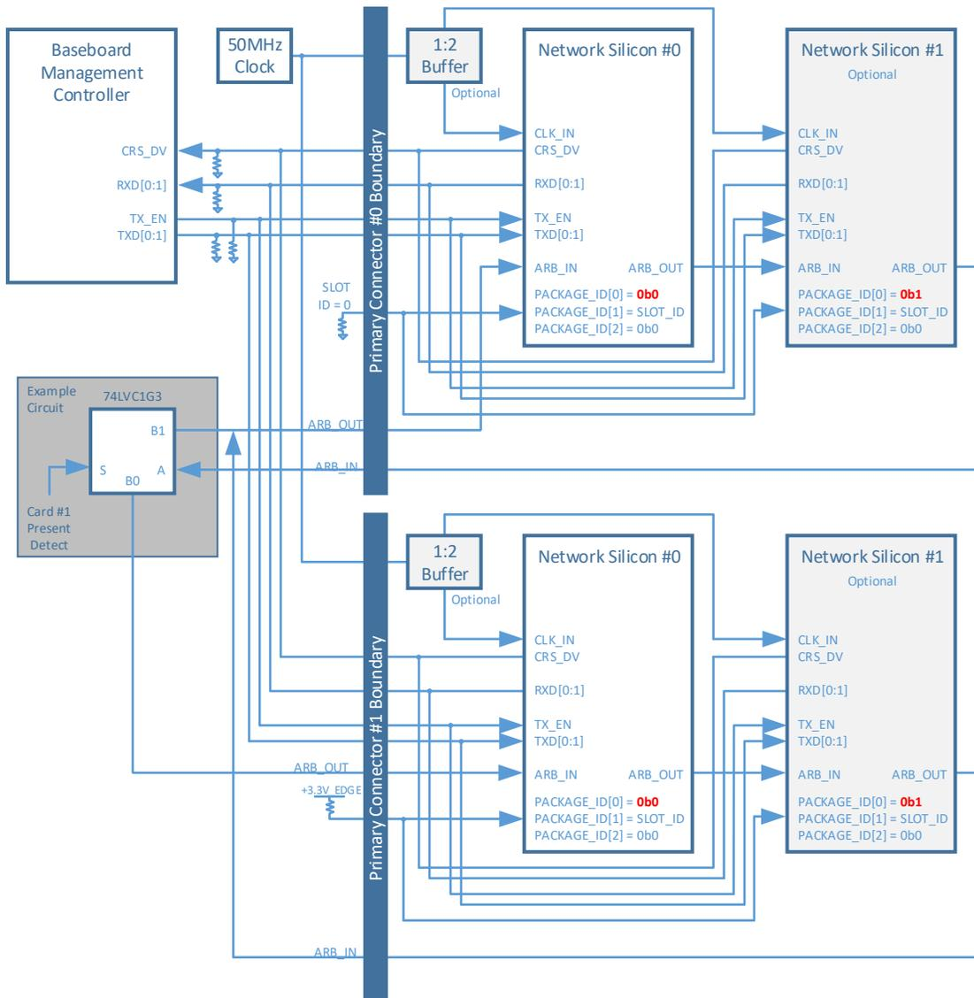
**Note 1:** For baseboard designs with a single Primary Connector, connect ARB\_IN to ARB\_OUT to complete the NC-SI hardware arbitration ring. For designs with multiple Primary Connectors, connect ARB\_IN and ARB\_OUT to an analog mux to complete the NC-SI arbitration ring based on the number of cards installed in the system. An example dual Primary Connector implementation is shown in Figure 80.
