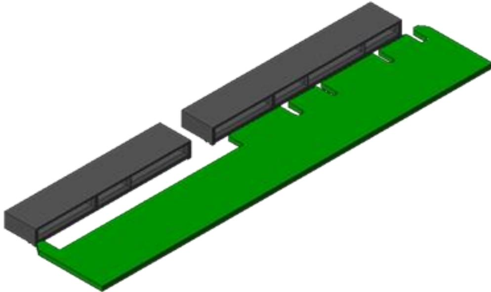
For both form-factors, an OCP NIC 3.0 card may optionally implement a subset of pins to support up to a x8 PCIe connection. This is implemented using a 2C card edge per SFF-TA-1002. The Primary Connector may support a 2C sized OCP NIC 3.0 card along with the 28 pin OCP bay shown in the 4C+ drawings. The following diagram from the SFF-TA-1002 specification illustrates the supported host Primary and Secondary Connectors and OCP NIC 3.0 card configurations.
