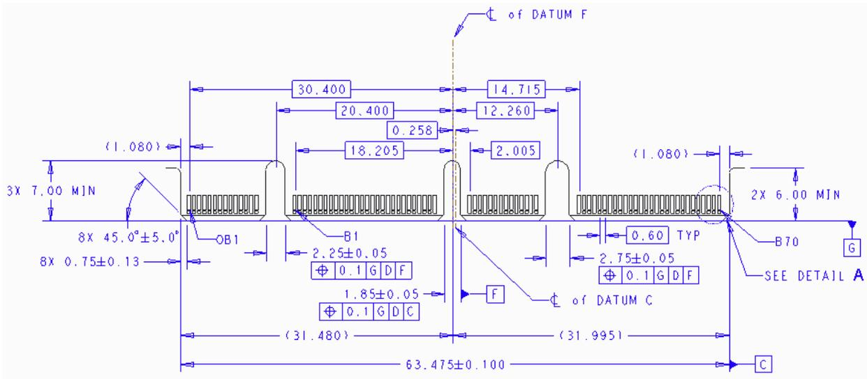
Figure 64: Large Size Card Gold Finger Dimensions – x32 – Top Side (“B” Pins)
