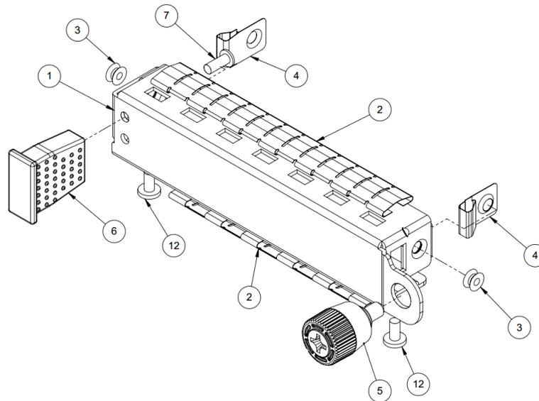
Figure 8: Small Card Standard I/O Bracket with Thumbscrew and Pulltab (2D View)
