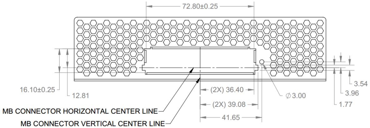
Figure 23: Small Form Factor Baseboard Chassis to Card Thumb Screw CTF Dimensions (Side View)
