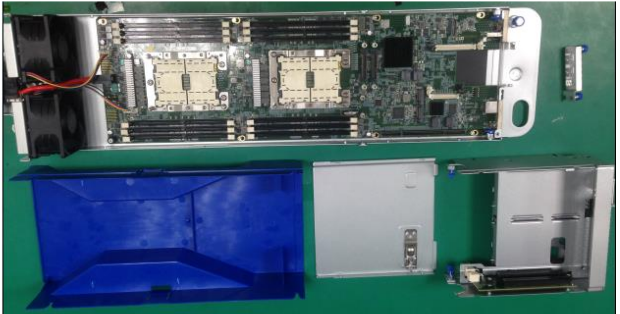
Figure 25 Server base mechanics, motherboard, air guide and front assembly
