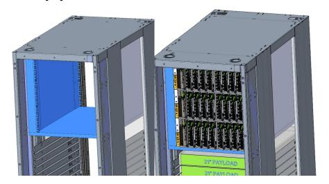
If shifting the system bus bar to Left-side or Right-side of the rack, there is enough remaining width for 19" rack subframe + 0.8" of budget for clearances and tolerances.
