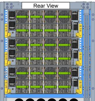
Enough horizontal space for **4-post 19" subframe** and outboard full-height 48V bus bar.
