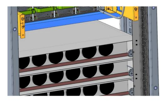
ORv3 Gear mounts similarly to ORv2 Gear when utilizing IT Gear Sled with Horizontal Bus Bar.
