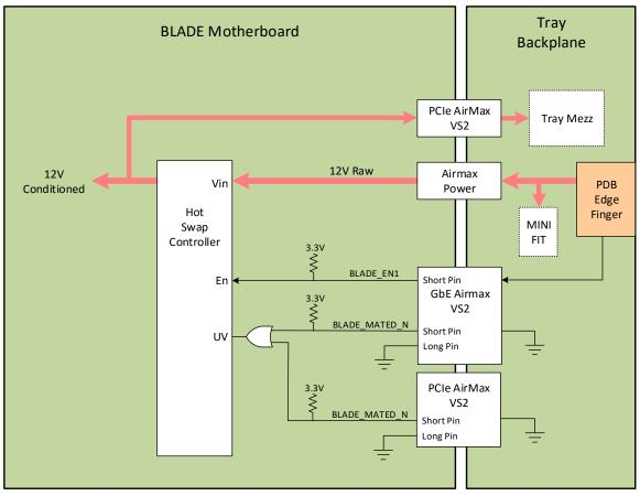
Figure 18: HSC functional block diagram
