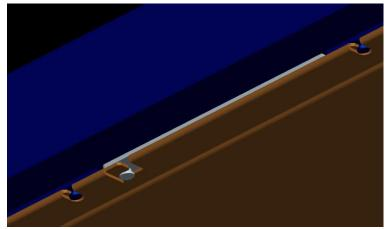
Figure 29. Example of a front-blade guide and latch
