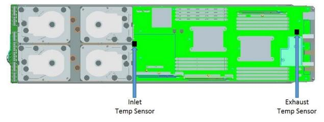
Figure 17: Temperature sensor locations
