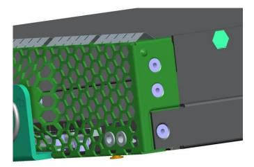
Figure 27: Front surface dimple
