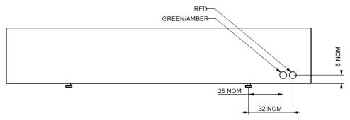
Figure 19: Front blade LED locations
