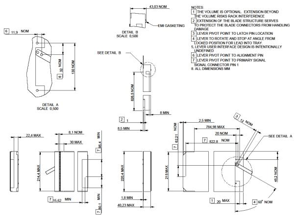
Figure 24: Dimensions of the volume that holds the blade
