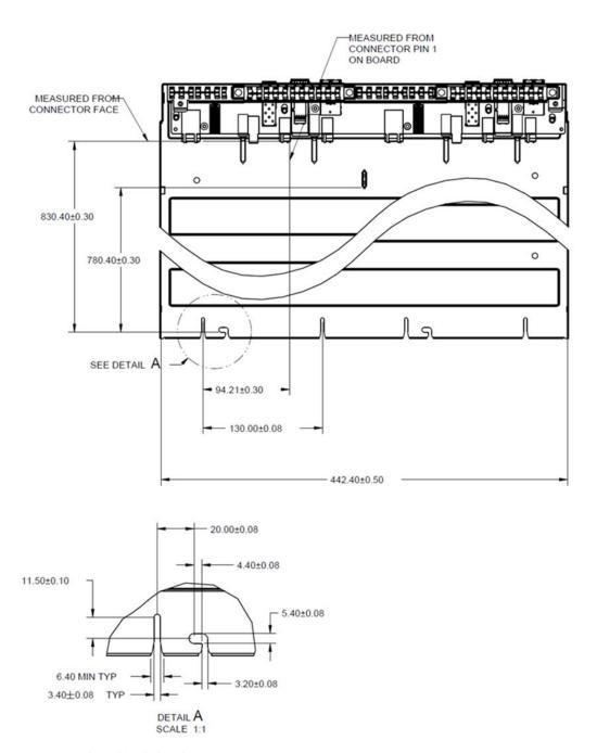
Figure 28: Guide and latch details, top view
