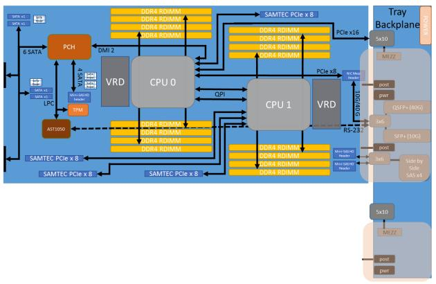
Figure 5: Baseline configuration of blade
