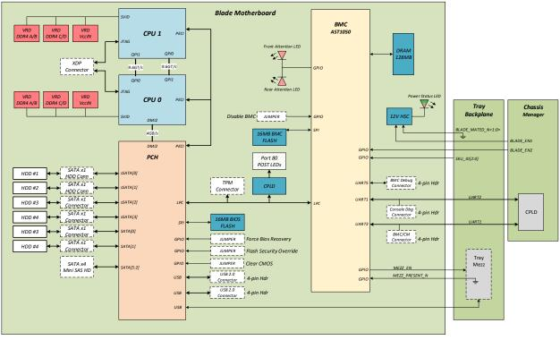
Figure 15: Blade management block diagram
