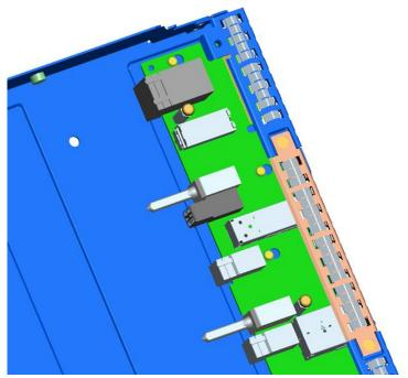
Figure 30: Example of a rear-blade guide pin
