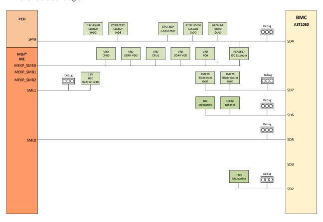
Figure 16: PCH / BMC I2C block diagram
