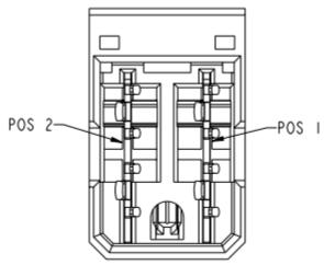
Figure 12: AirMax power receptacle pinout arrangement
