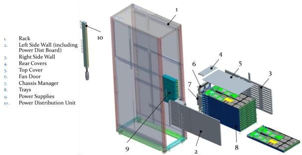
Figure 1: View of OCS with rack
