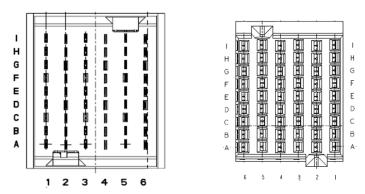
Figure 14: AirMax VS2 pinout arrangement
