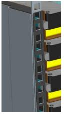
Figure 8: Column air flow passage
