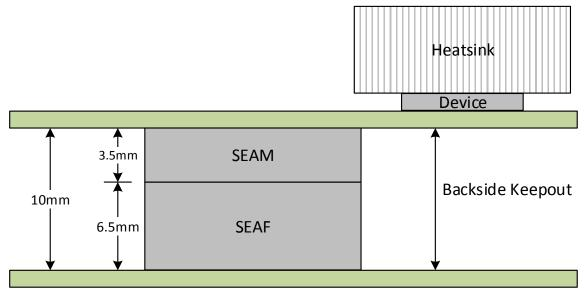
Figure 2. Connector stackup
