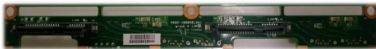
Figure 13. Storage HDD backplane board, side 2
