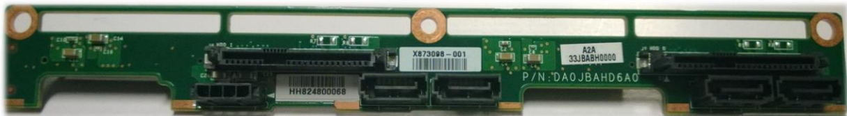
Figure 12. Storage HDD backplane board, side 1
