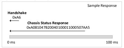
Figure 10. Message payload encapsulated with the serial start and stop bytes
