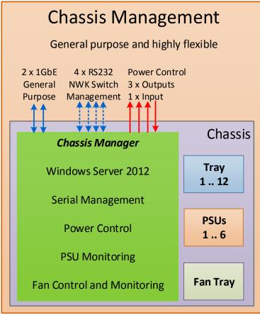
Figure 2. Top level representation of chassis manager
