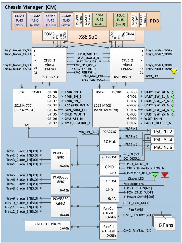
Figure 3. Chassis manager hardware block diagram
