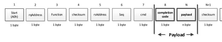
Figure 11. Chassis manager payload
