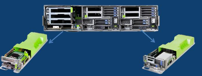
High Performance Compute Blade Intel<sup>®</sup>Xeon<sup>®</sup> Skylake SP family <u>1x LFF drive with 2x FH PCIe slots</u>
