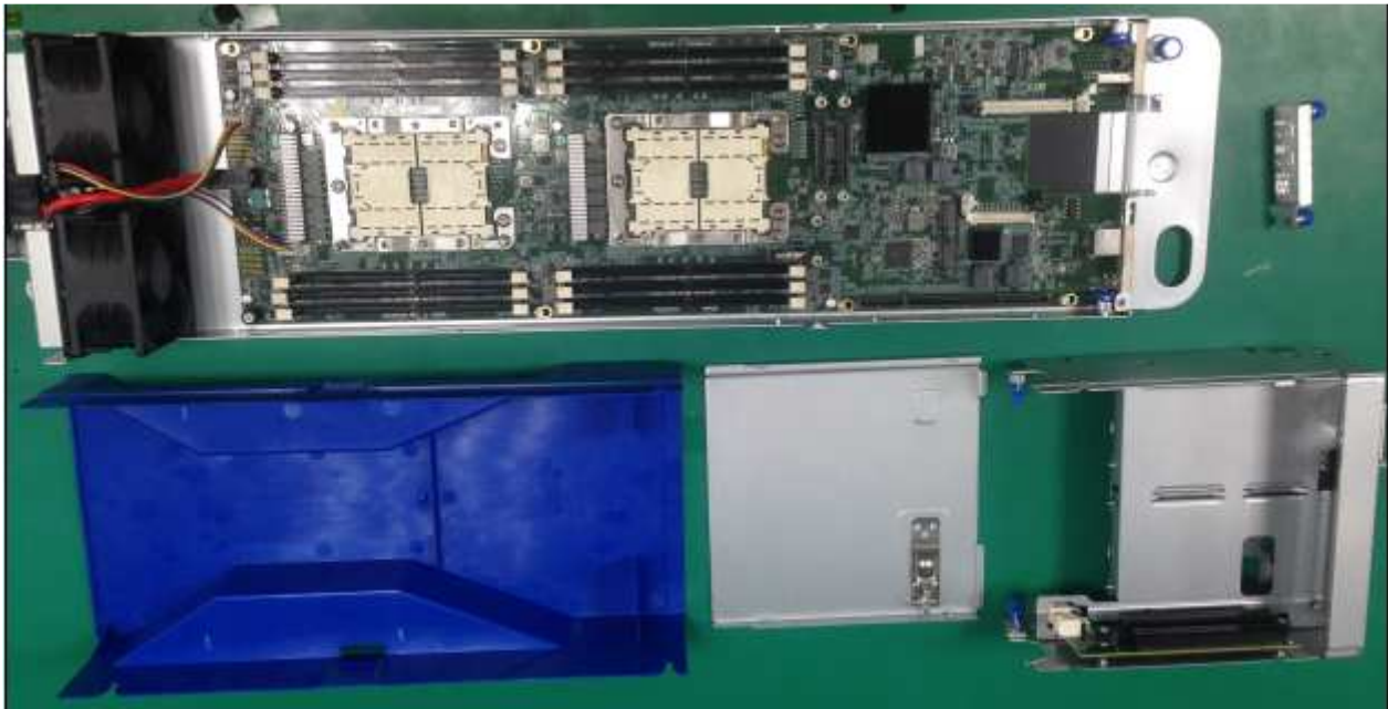
Figure 25 Server base mechanics, motherboard, air guide and front assembly
