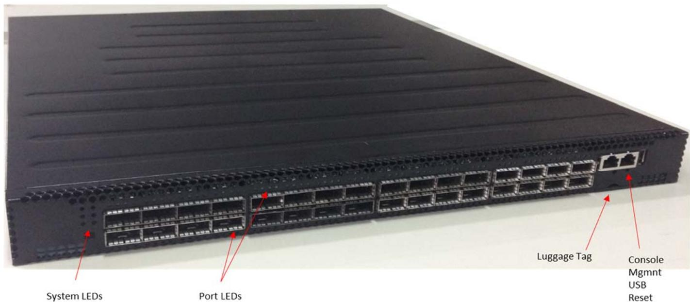
The front panel view of the AS7500-32X includes the following key components:
