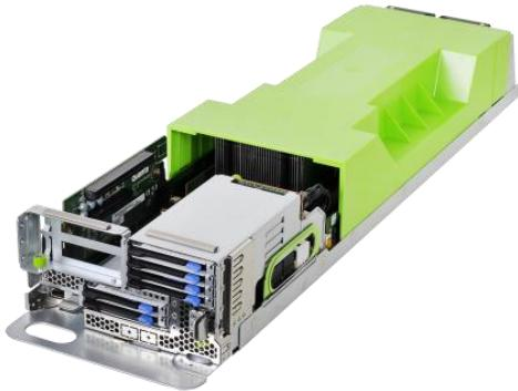
Figure 3 2x HH Slots with 6x2.5" HDD SKU(Single Side)
