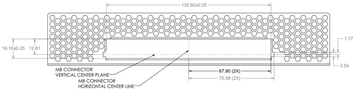
Figure 53: LFF Baseboard Chassis CTF Dimensions (Side View)
