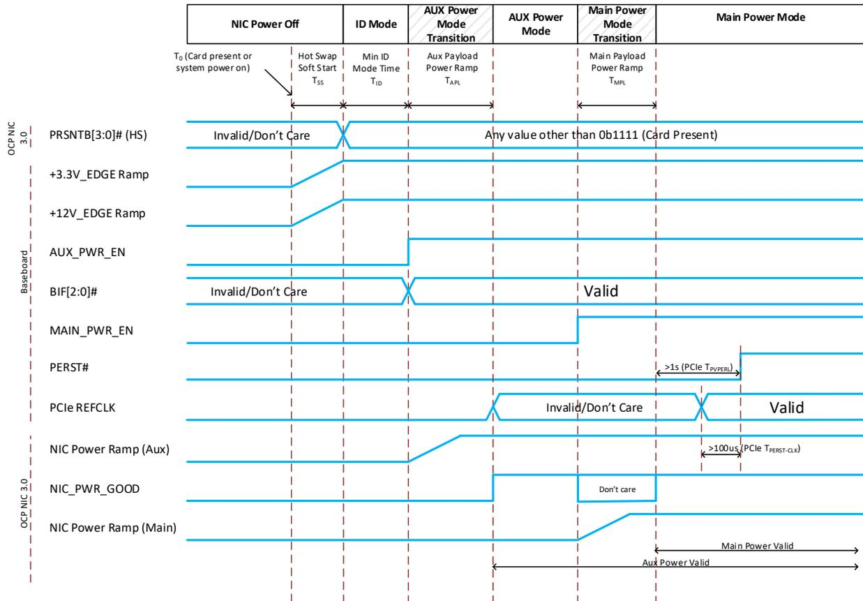
Figure 95: Power-Down Sequencing
