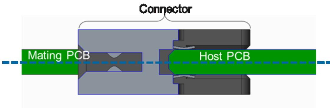
Figure 71: 0.3mm Offset for 0.076" Thick Baseboards
