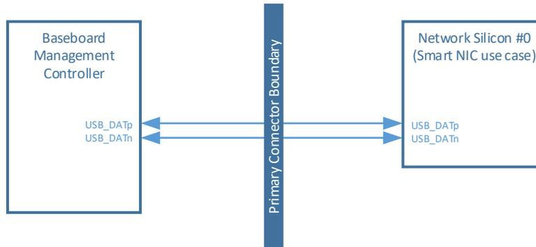
Figure 83: USB 2.0 Connection Example – USB-Serial / USB-JTAG Connectivity
