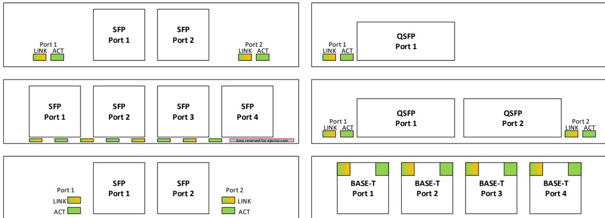
Note 1: The example port and LED ordering diagrams shown in Figure 92 are viewed with the card in the horizontal position and the primary side is facing up.
