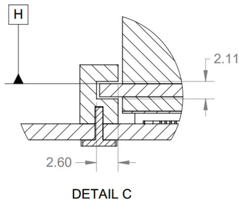
The right angle and straddle mount card guides are identical between the Small and Large form factor cards. The card guide models are included in the 3D CAD packages and may be downloaded from the OCP NIC 3.0 Wiki site: <http://www.opencompute.org/wiki/Server/Mezz>.
