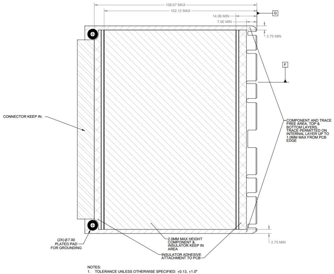
Figure 32: LFF Keep Out Zone – Side View
