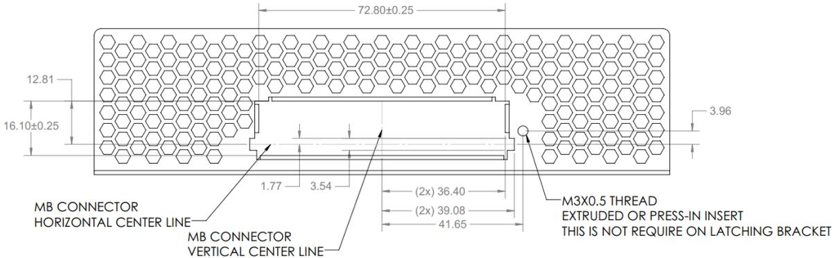
Figure 45: SFF Baseboard Chassis to Card Thumb Screw CTF Dimensions (Side View)
