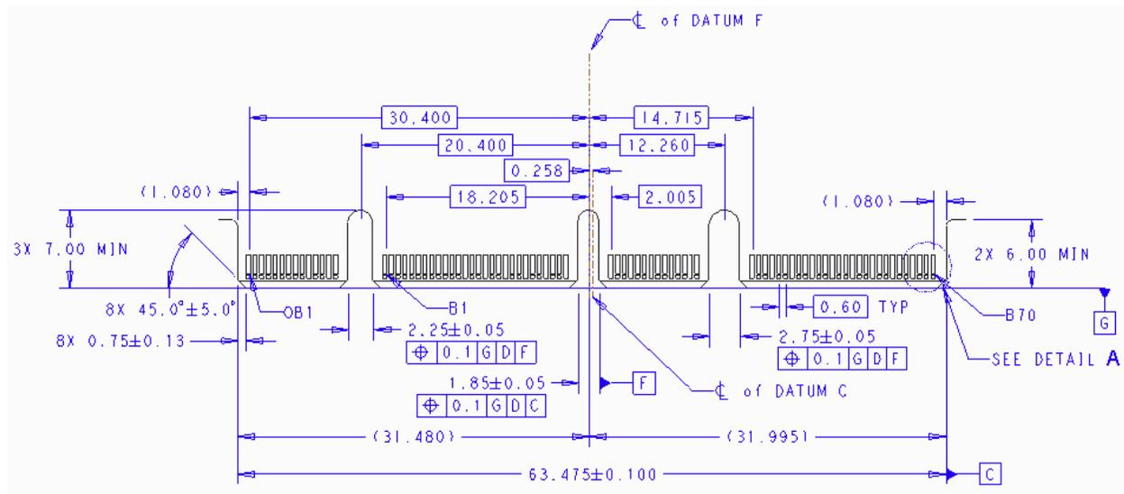
Figure 62: LFF Gold Finger Dimensions – x32 – Top Side (“B” Pins)
