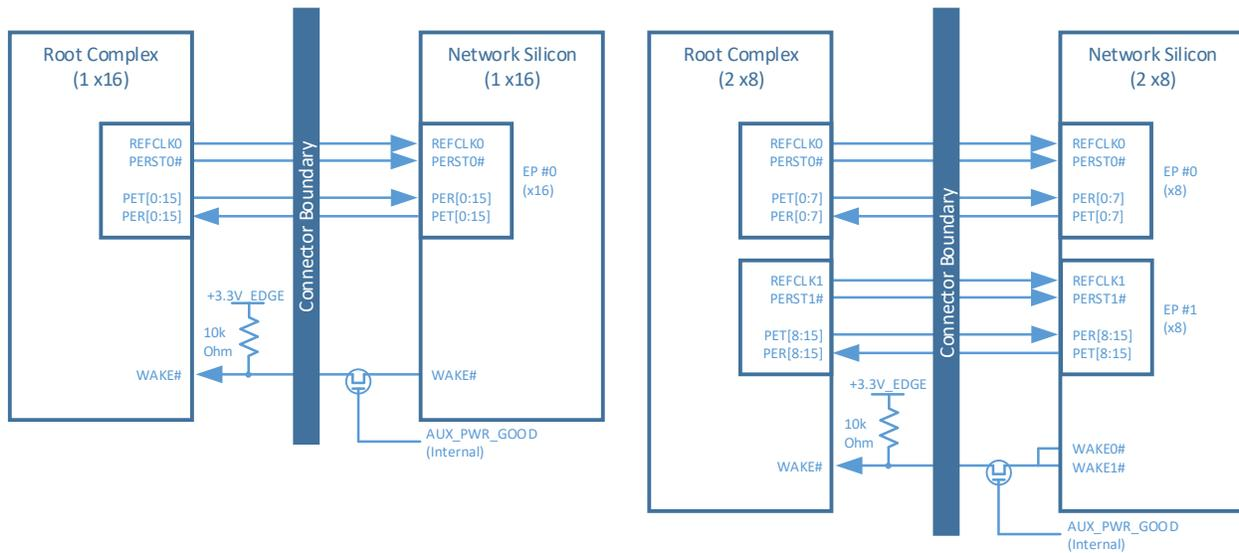
Figure 91: PCIe Interface Connections for a 4 x4 OCP NIC 3.0 Card
