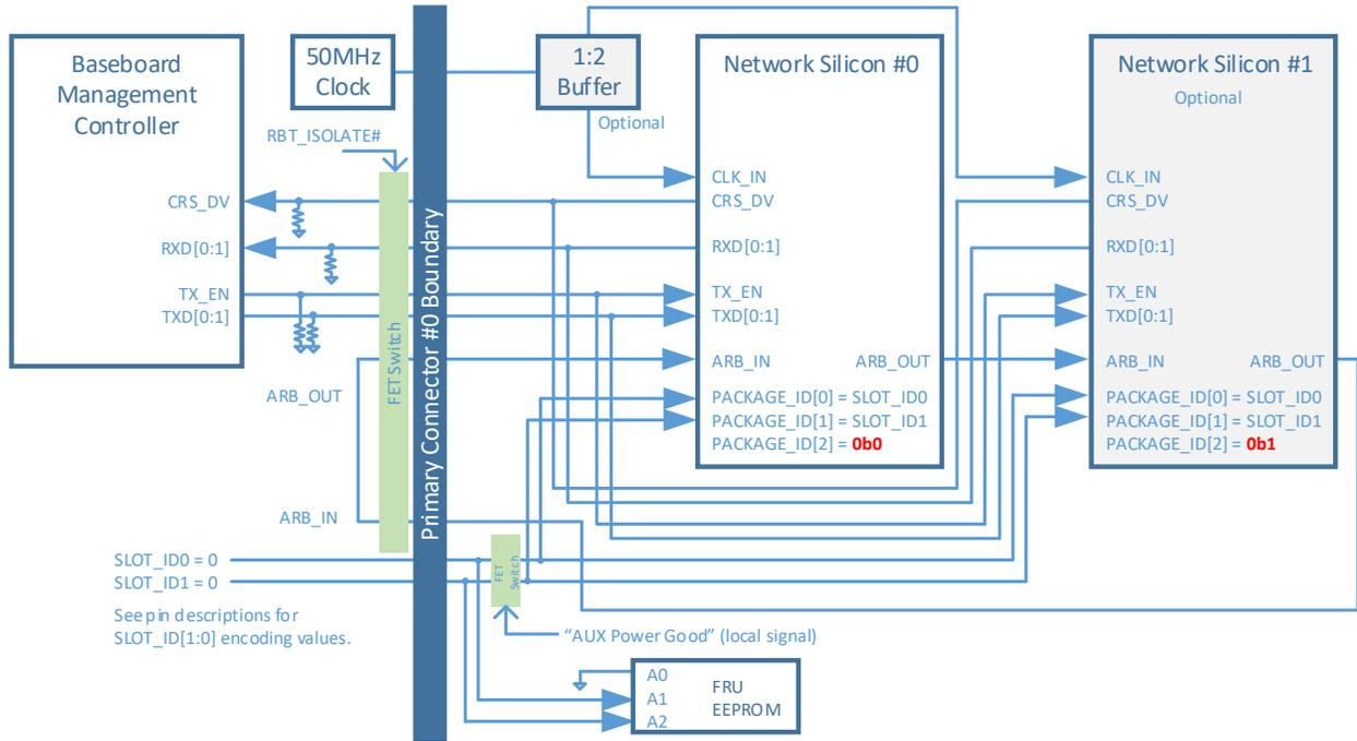
Figure 78: NC-SI Over RBT Connection Example – Dual Primary Connectors
