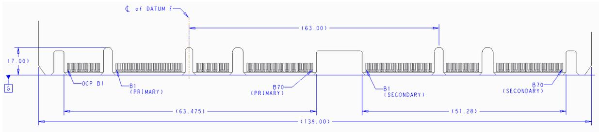
Figure 63: LFF Gold Finger Dimensions – x32 – Bottom Side (“A” Pins)
