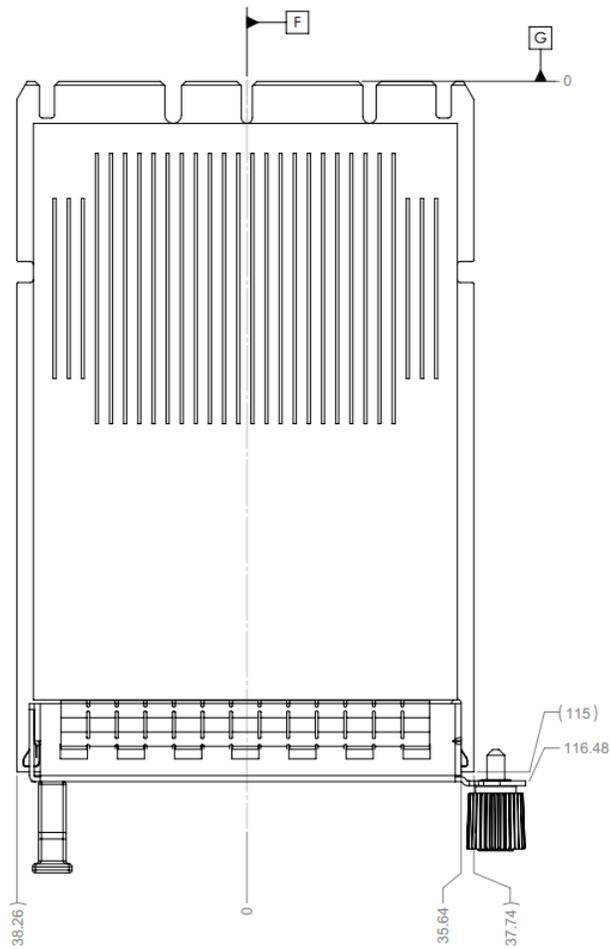
Figure 39: SFF OCP NIC 3.0 Card with Pull Tab CTF Dimensions (Front View)
