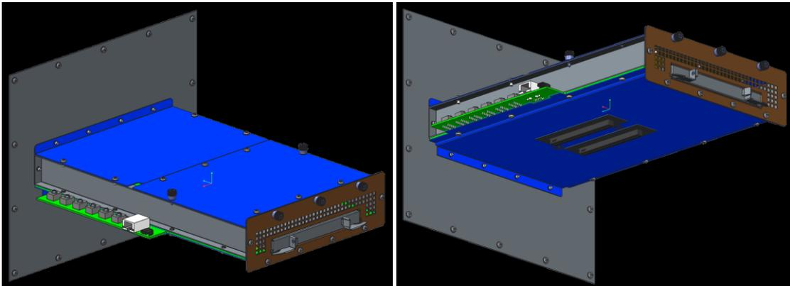
Figure 116: LFF Card Thermal Test Fixture Design – Cover Removed
