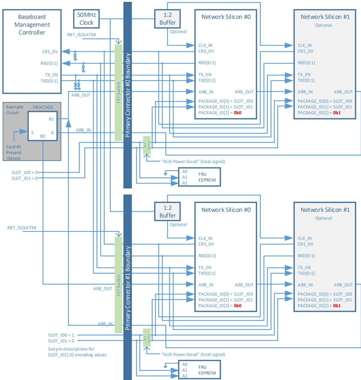
**Note 1:** For baseboard designs with a single Primary Connector, connect ARB\_IN to ARB\_OUT to complete the NC-SI hardware arbitration ring. For designs with multiple Primary Connectors, connect ARB\_IN and ARB\_OUT to an analog mux to complete the NC-SI arbitration ring based on the number of cards installed in the system. An example dual Primary Connector implementation is shown in Figure 78.
