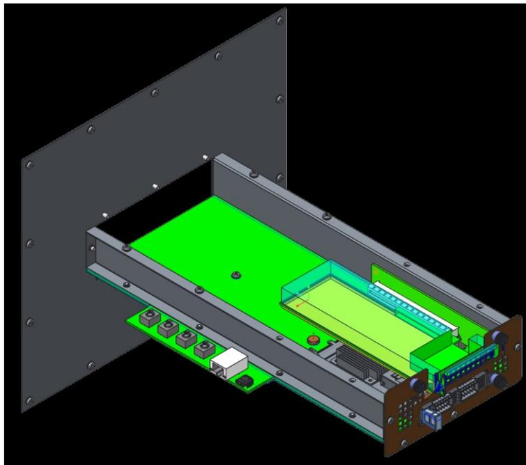
Figure 114: SFF Card Thermal Test Fixture PCB
