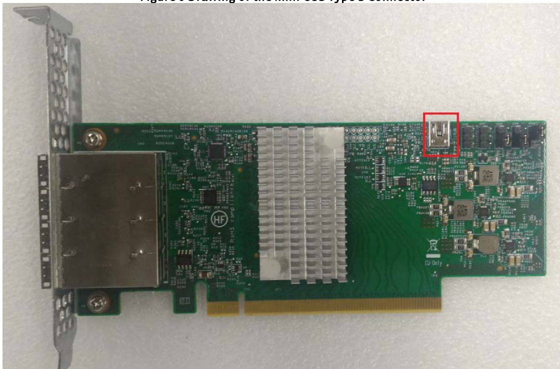
Figure 7 Location of the Mini-USB Type B Connector on a Retimer Card
