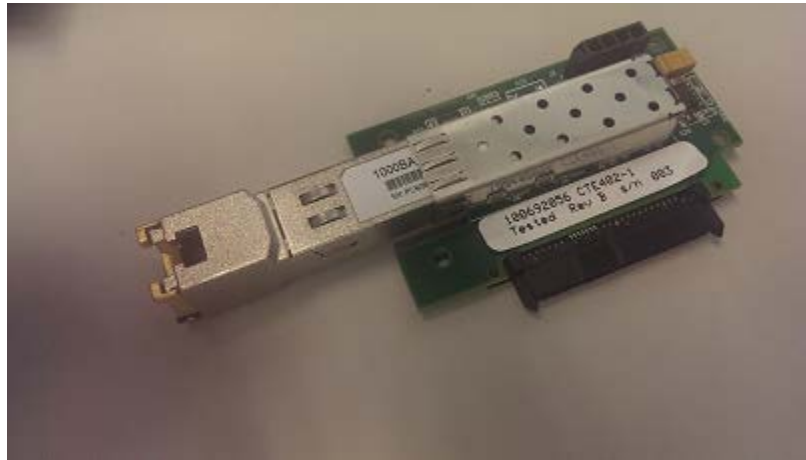
Figure 5 SFP module installation
