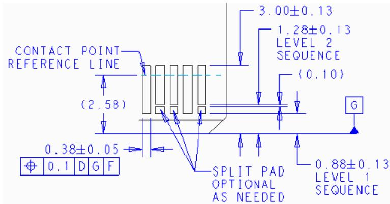
Figure 69: LFF Gold Finger Dimensions – x32 – Top Side (“B” Pins)
