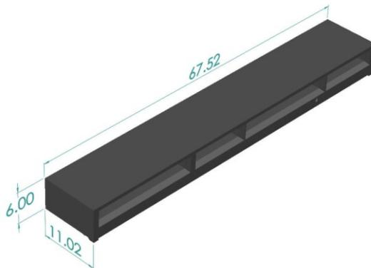
Figure 72: 140-pin Base Board Secondary Connector – Right Angle
