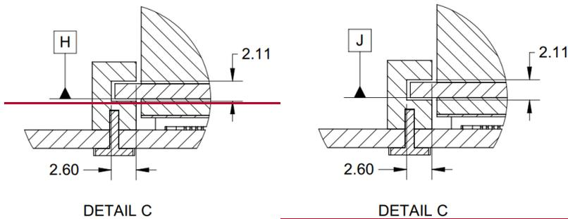
The right angle and straddle mount card guides are identical between the SFF and LFF. The card guide models are included in the 3D CAD packages and may be downloaded from the OCP NIC 3.0 Wiki site: <http://www.opencompute.org/wiki/Server/Mezz>.
