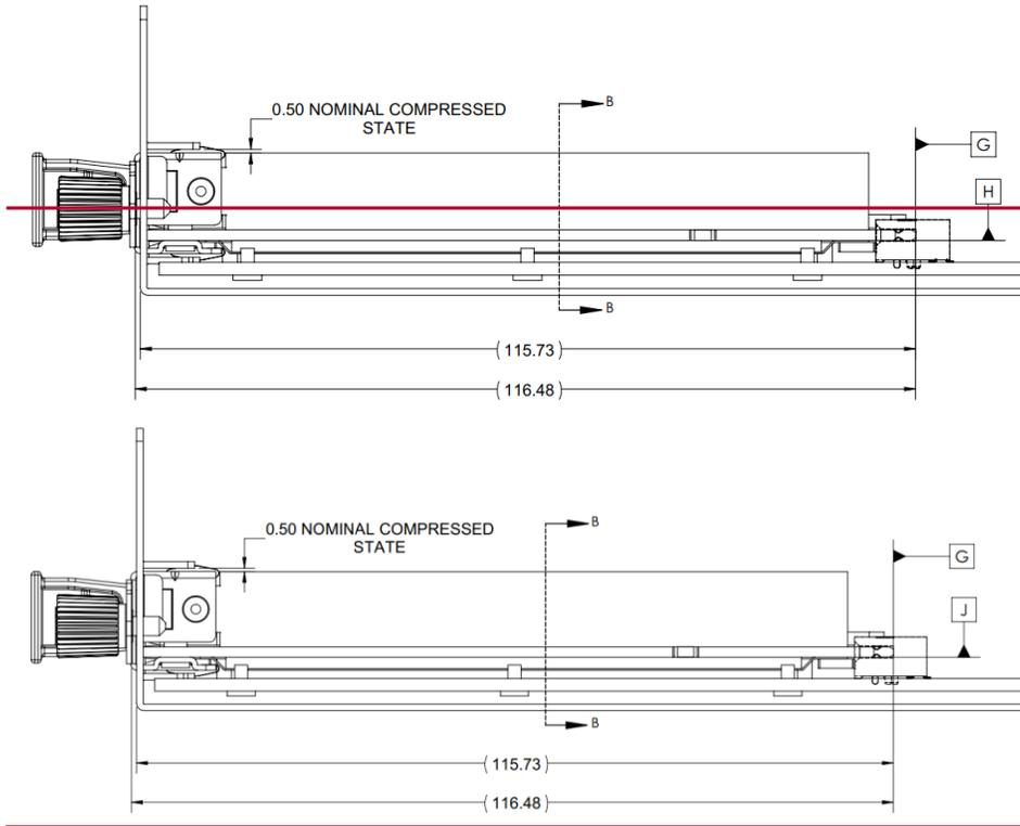
Figure 51: SFF Baseboard Chassis to Ejector lever Card CTF Dimensions (Side View)
