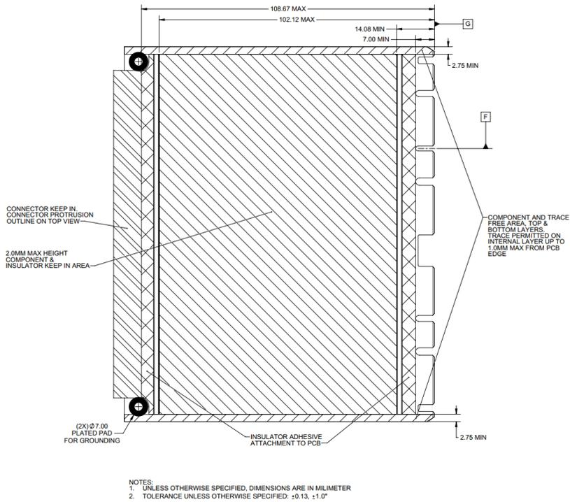
Figure 32: LFF Keep Out Zone – Side View
