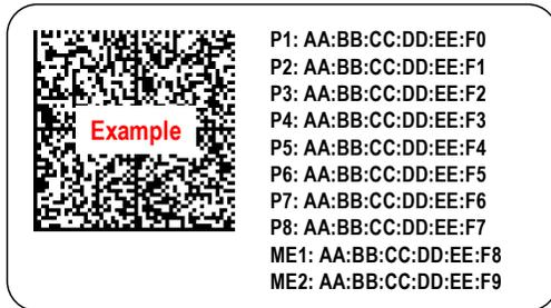
**2.9.2.3 MAC Address Label Example 3 – Quad Port with Dual Hosts, Dual Managed Controllers**
