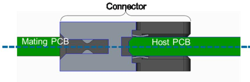
Figure 78: 0.3 mm Offset for 0.076" Thick Baseboards
