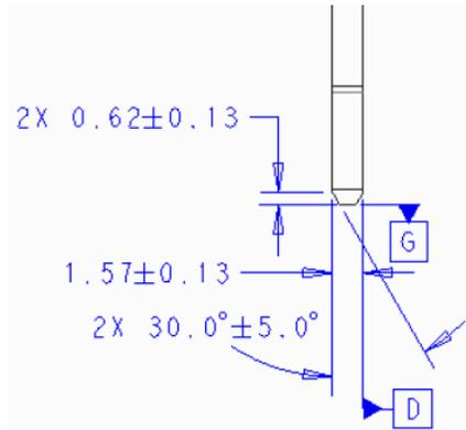
Figure 68: SFF Primary Connector Gold Finger - Detail D
