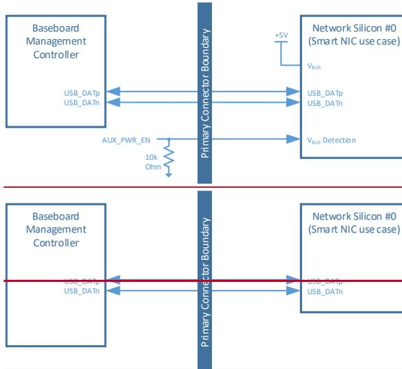
Figure 90: USB 2.0 Connection Example – USB-Serial / USB-JTAG Connectivity
