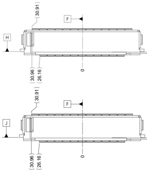
Figure 45: SFF OCP NIC 3.0 Card with Ejector CTF Dimensions (Side View)
