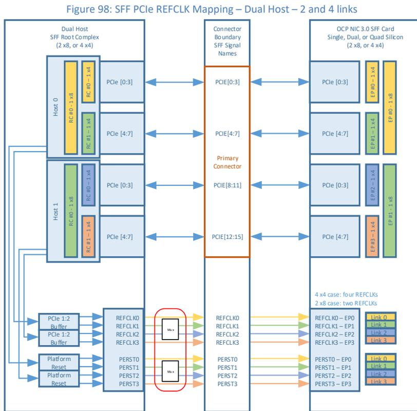
**Note:** For dual host applications that connect to a two link endpoint, the baseboard Host 1 REFCLK0 and PERST0 signal needs to be multiplexed to the REFCLK1 and PERST1 pins of the OCP NIC 3.0 card edge. This ensures the mandated Link n, REFCLKn and PERSTn mappings are maintained.
