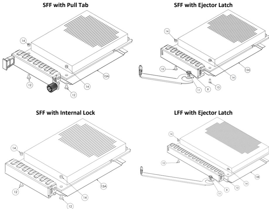
Diagram callouts #8, and #11 through #15 are installed at the NIC assembly level:
