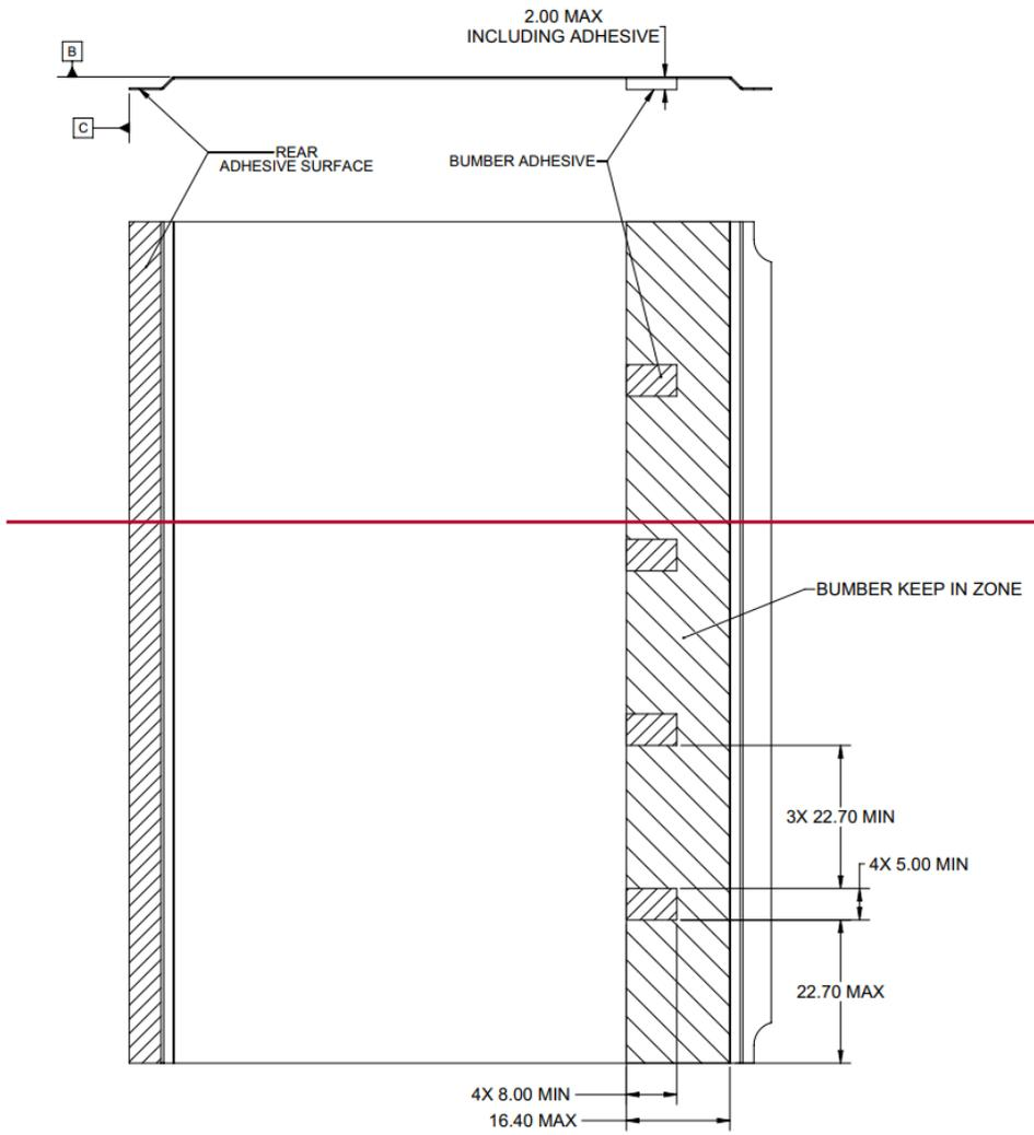
ALTERNATE OPTION USING BUMPER & ADHESIVE FOR ATTACHING THE INSULATOR TO PCB INSTEAD OF USING FRONT ADHESIVE SURFACE.
