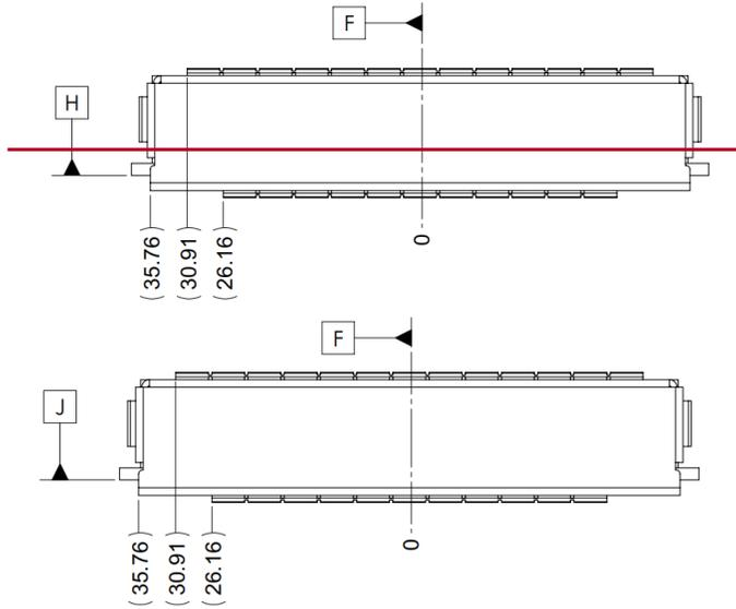
Figure 48: SFF OCP NIC 3.0 Card with Internal Lock CTF Dimensions (Side View)
