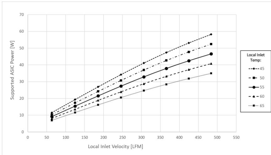
The curves shown in Figure 115 were obtained using CFD analysis of the reference OCP NIC 3.0 LFF card. The reference card has a 45 mm x 45 mm ASIC with two QSFP connectors. Additional card geometry parameters and boundary conditions used in the reference CFD analysis are summarized in Table 60. Figure 116 shows a comparison of the 3D CAD and CFD model geometry for the reference OCP NIC 3.0 card.
