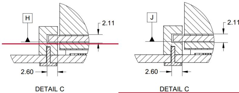
The right angle and straddle mount card guides are identical between the SFF and LFF cards. The card guide model is included in the 3D CAD packages and may be downloaded from the OCP NIC 3.0 Wiki site: <http://www.opencompute.org/wiki/Server/Mezz>.
