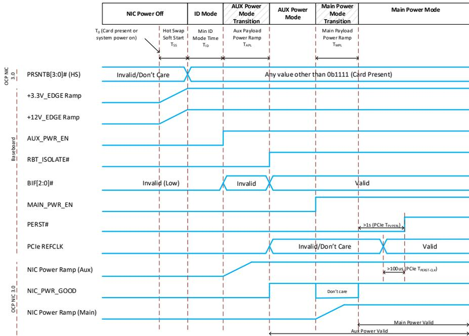
Note 1: The RBT isolation state is controlled with the baseboard RBT\_ISOLATE# signal. This controls the baseboard RBT isolator.
