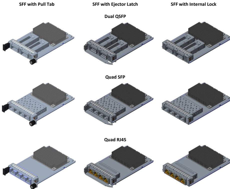
Figure 9 illustrates example SFF 3D views of the pull tab and ejector latch assemblies mounted in a chassis utilizing a straddle mount connector and a right angle connector. The baseboard connector options are discussed in Section 3.2. The SFF OCP NIC 3.0 card is identical for both chassis connector options.
