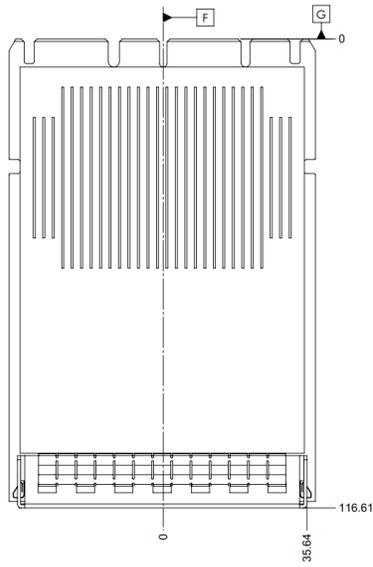
Figure 47: SFF OCP NIC 3.0 Card with Internal Lock CTF Dimensions (Front View)
