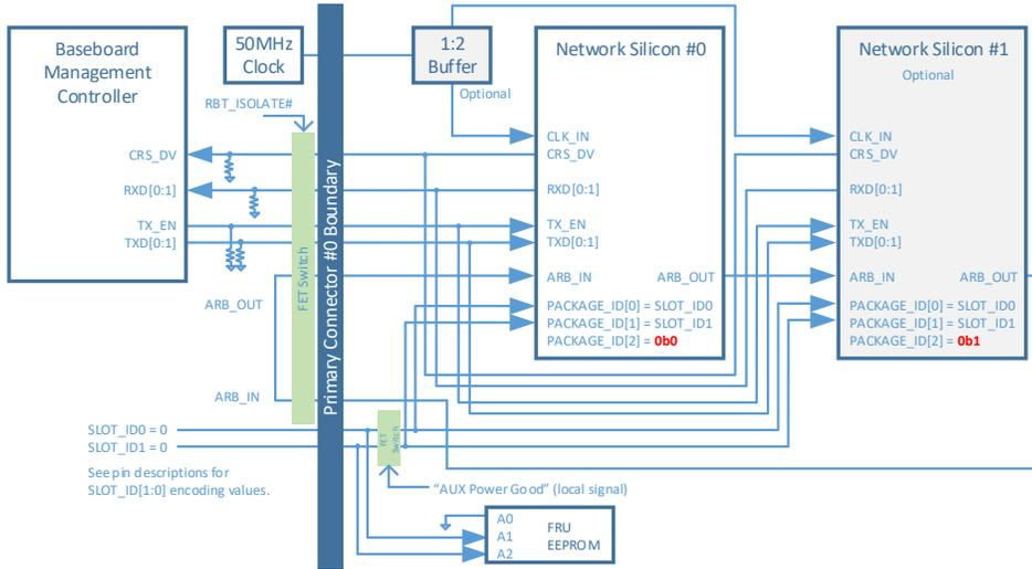
**Note 3:** The logical implementation of the hardware arbitration ring shall maintain the arbitration ring integrity when there exists one or more cards that are plugged in, but are powered off (e.g. in ID Mode).
