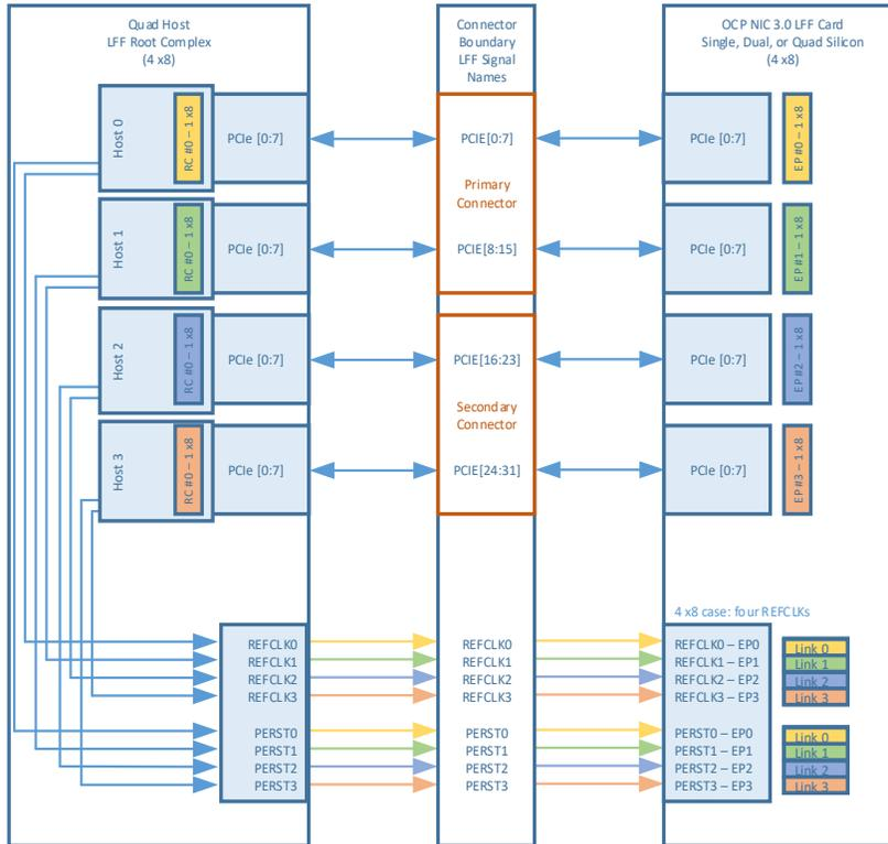
**Note:** For quad host applications that connect to a two link endpoint, the baseboard Host 2 REFCLK and PERST signal needs to be multiplexed to the REFCLK1 and PERST1 pins of the OCP NIC 3.0 card edge. This ensures the mandated Link  $n$ , REFCLK $n$  and PERST $n$  mappings are maintained.
