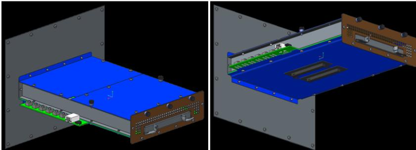
Figure 128: LFF Card Thermal Test Fixture Design – Cover Removed
