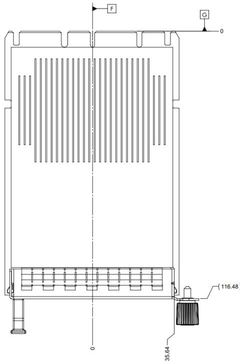
Figure 41: SFF OCP NIC 3.0 Card with Pull Tab CTF Dimensions (Front View)
