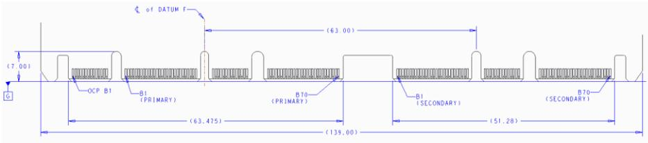
Figure 70: LFF Gold Finger Dimensions – x32 – Bottom Side (“A” Pins)
