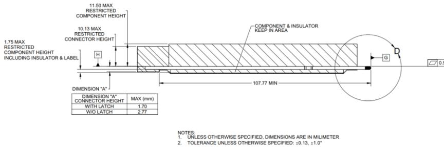
**Note:** The area defined by DIMENSION "A" is between the faceplate and the primary side of the board. Grounded through-hole mounting pins are permitted but should avoid making contact with the latching mechanism and EMI fingers. Signal pins are not permitted in this area.
