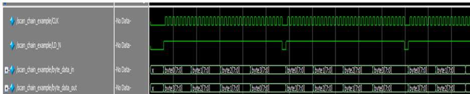
The scan chain provides sideband status indication between the OCP NIC 3.0 card and the baseboard. The scan chain bit definition is defined in the two tables below. The scan chain data stream is 32-bits in length for both the DATA\_OUT and the DATA\_IN streams. The scan chain implementation is optional on
