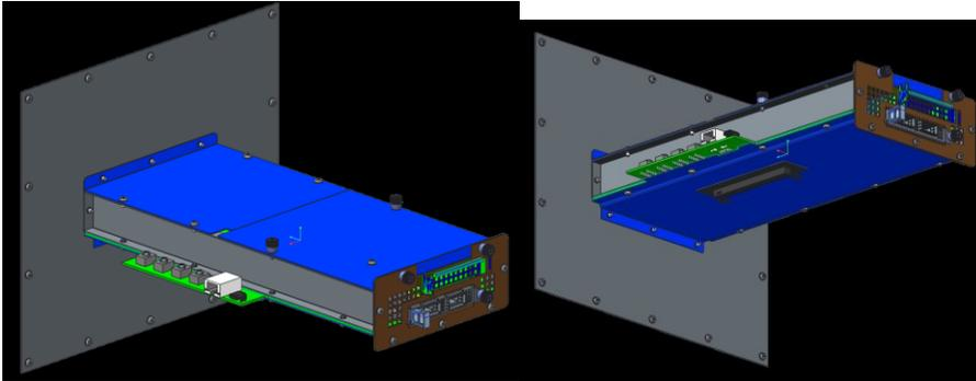
Figure 125: SFF Thermal Test Fixture Preliminary Design – Cover Removed
