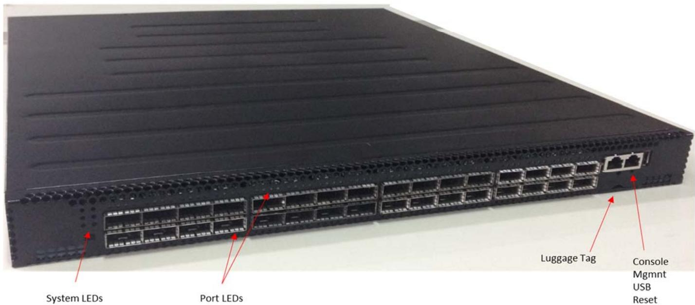
The front panel view of the AS7712-32X includes the following key components:
