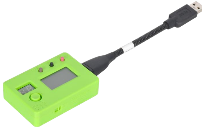
Figure 1 QCT Rackgo X OCP Debug Card with LCD
