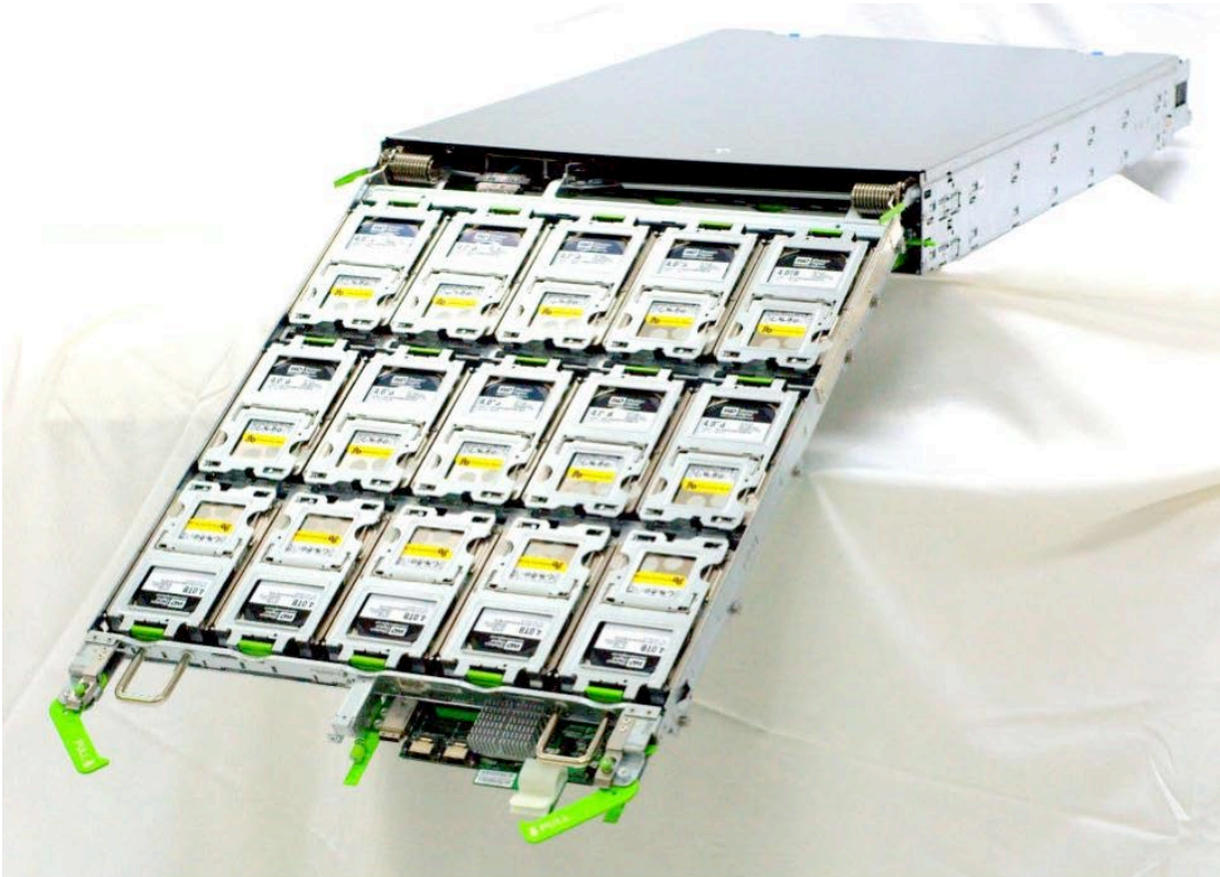
Figure 2 Open Vault Detail Showing the Hinged Disk Drive Tray
