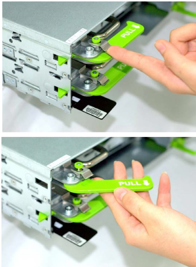
Figure 61 HDD Tray/Chassis Cam Latches
