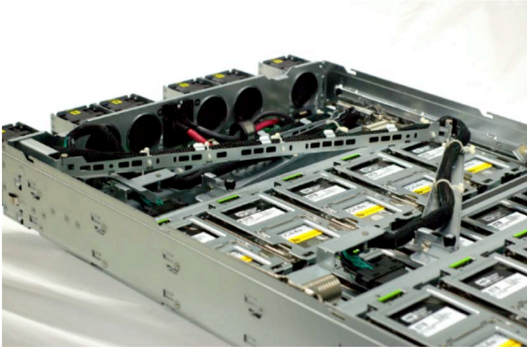
Figure 68 HDD Tray Cable Arm
